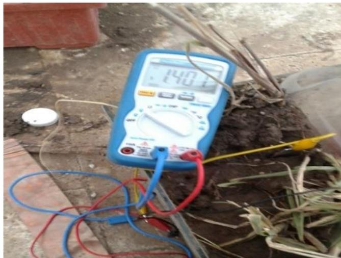
We tested two types of proton exchange membrane (PEM): (Nylon) and (Gelatin). We recorded the voltage of the P-MFC using these new (PEM) over 4 times a day. And the results were:
