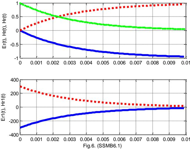
Thus, the solution of the Maxwell equations for a capacitor being charged and the solution for a capacitor in a sinusoidal current circuit differ only in that the former includes exponential time functions while the latter contains sinusoidal time functions.
