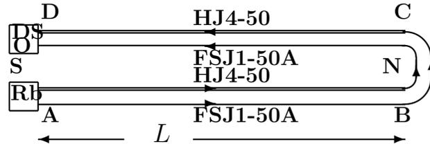
Figure 5: Because Fresnel drag is absent in RF coaxial cables this dual cable setup, using one clock, is capable of detecting the absolute motion of the detector wrt to space, revealing the sidereal rotation effect as well as wave/turbulence effects. The cables in each circuit are configured into 8 loops, as in Fig.6, giving  $L = 8 \times 1.85\text{m} = 14.8\text{m}$ .
