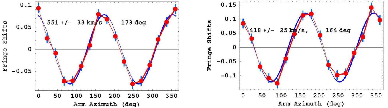
Figure 4: Examples of detected fringe shifts from rotation after removing the temperature and non-orthogonal mirror effects from the data. Left: Michelson-Morley fringe shifts, from 1887. Right: Miller interferometer fringe shifts 1925/26. Plots show both data and expected  $\cos(2(\theta - \psi))$  form in (2). Error bars show rms deviation between these.
