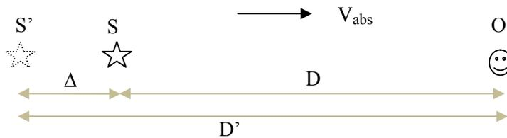
The source appears to have shifted away from the observer by distance  $\Delta$ . The observer  $O$  measuring the time delay  $T$  between emission and detection of the light pulse will be able to make correct explanation and prediction only by assuming that the light pulse started from  $S'$  and not from  $S$ , and by assuming that the speed of light is equal to  $c$  relative to the apparent source  $S'$ .
