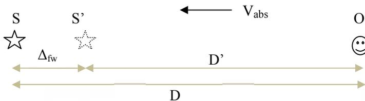
$$D' = D \frac{c}{c + V_{abs}} = 2 R \frac{c}{c + V_{abs}} \quad \text{and} \quad \Delta_{fw} = D \frac{V_{abs}}{c + V_{abs}}$$
