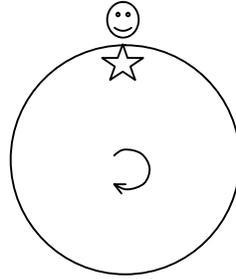
Assume that the light source emits light in the opposite directions tangentially. The two light beams travel in circular paths in opposite directions before being detected at the detector. A circular mirror is used to make light travel in circular path.
