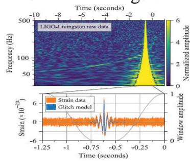
FIG. 2. Mitigation of the glitch in LIGO-Livingston data. Times are shown relative to August 17, 2017 12:41:04 UTC. *Top panel:* A time-frequency representation [65] of the raw LIGO-Livingston data used in the initial identification of GW170817 [76]. The
