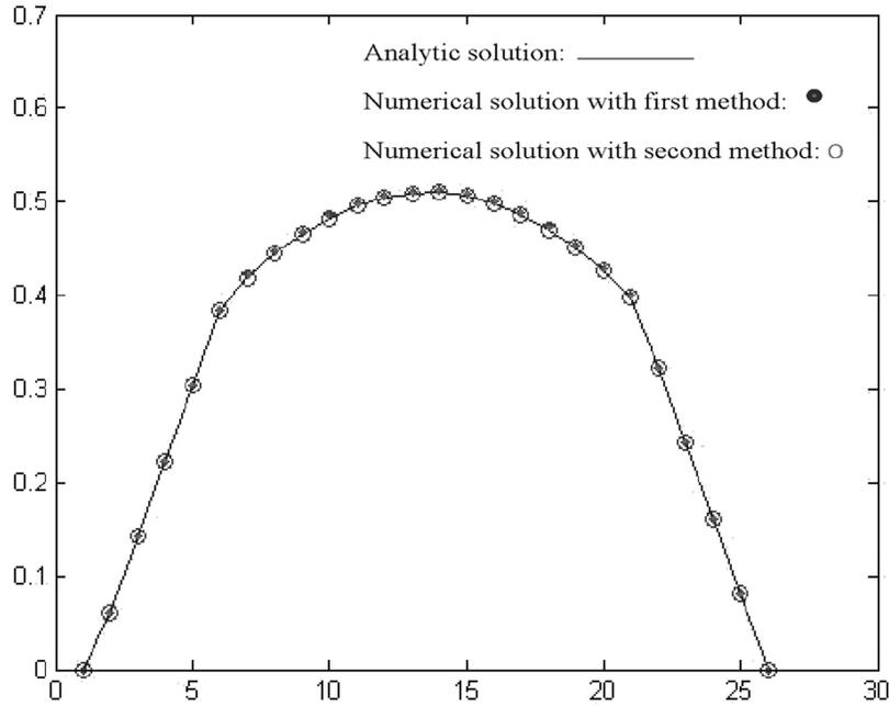
Figure 2: raphs of approximate and exact solutions of the partial differential equation (1) with two methods at  $\Delta t = 0.0317, \Delta x = \pi/99, h = 0.5$
