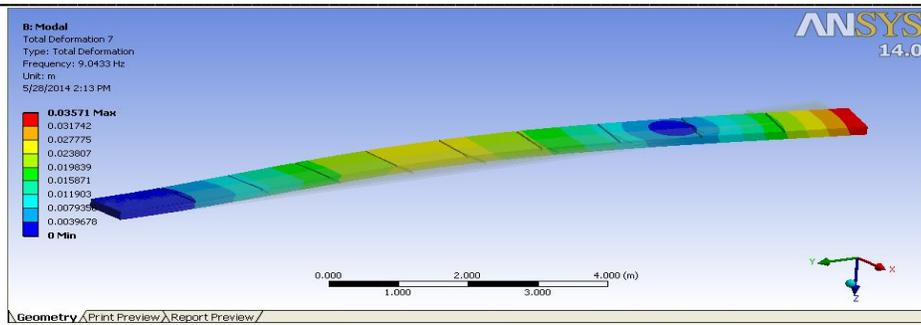
Figure 7 Fifth mode shape of composite Nylon beam with natural frequency 9.0433Hz
