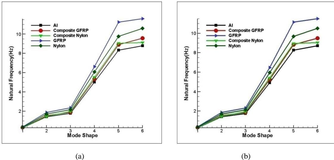
Figure 2 Variation between Natural frequency and Mode Shape (a) 0 Crack (b) 9 Cracks
