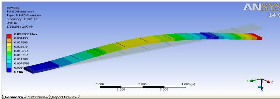
Figure 4 Second mode shape of composite Nylon beam with natural frequency 1.9378Hz
