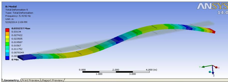
Figure 5 Third mode shape of composite Nylon beam with natural frequency 5.4192Hz
