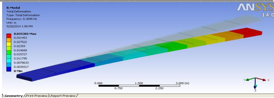
Figure 3 First mode shape of composite Nylon beam with natural frequency 0.3095Hz
