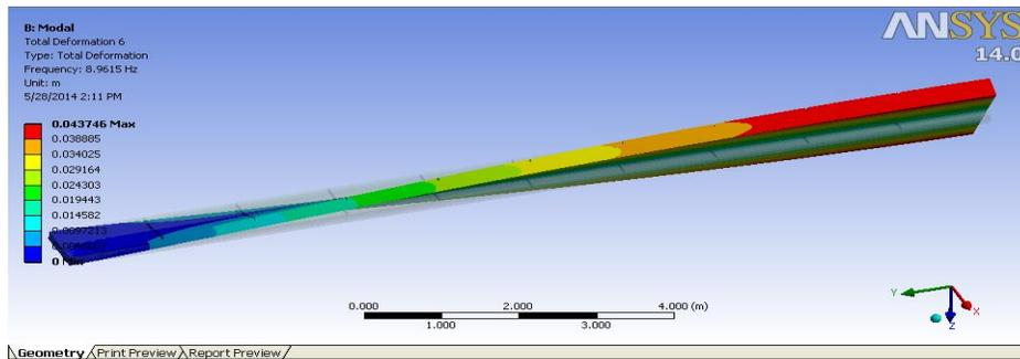
Figure 6 Fourth mode shape of composite Nylon beam with natural frequency 8.9615Hz
