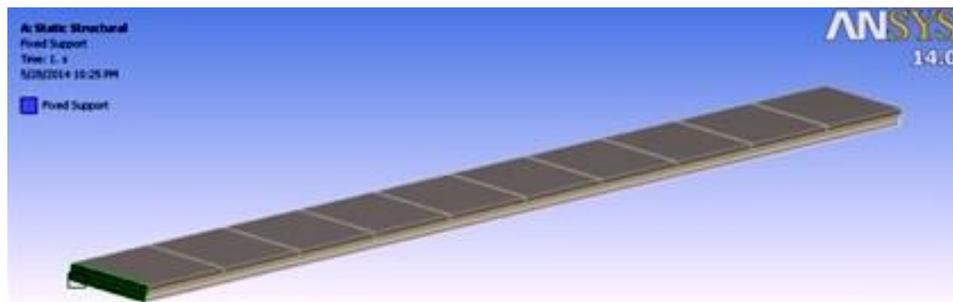
Figure 1 Mathematical Model of Composite Sandwich beam
