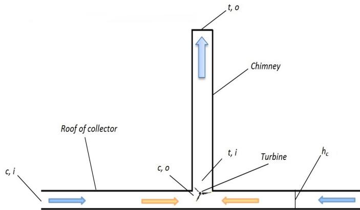
Figure 1: Schematic of SSCP with the applied variables and subscripts in the present analysis
