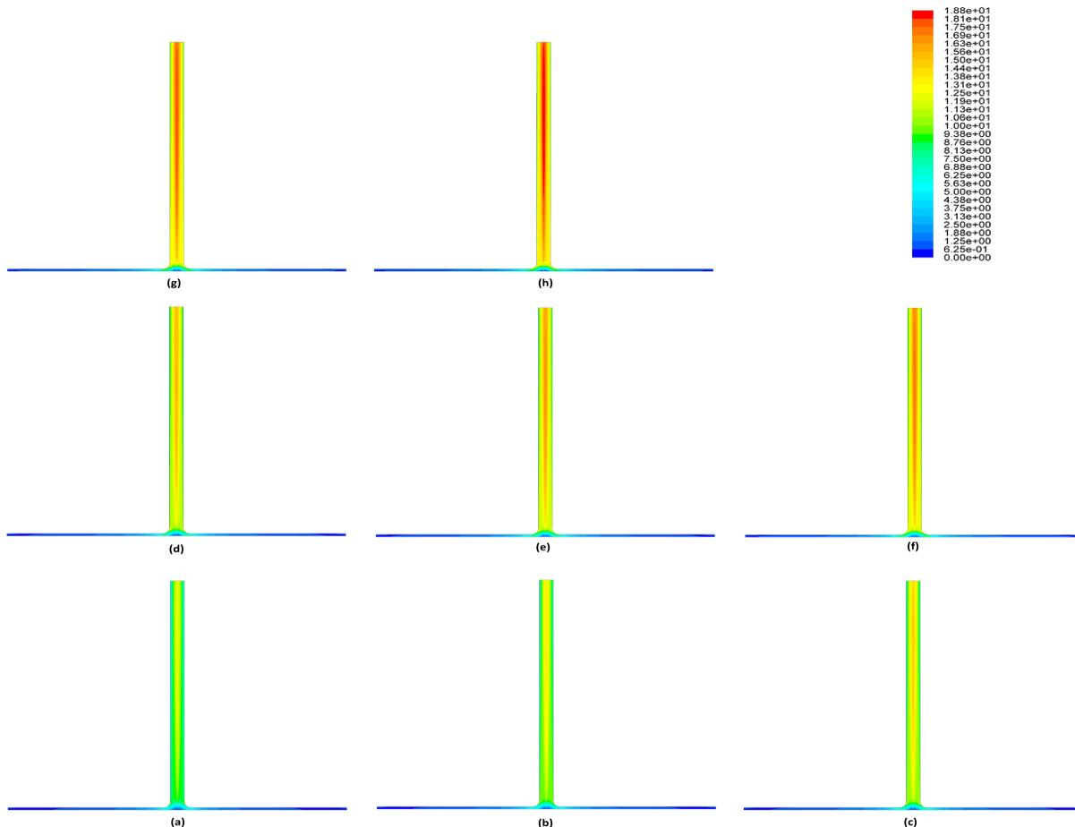
Figure 4: Velocity contour plot ( $m/s$ ) for different available solar heat flux at the ground of collector, (a):300, (b):400, (c):500, (d):600, (e):700, (f):800, (g):900, (h):1000  $W/m^2$ .
