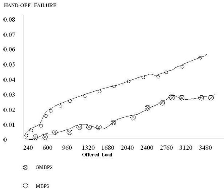
Fig. 3.(b) Graph showing the comparison of Guarded and non-Guarded schemes for Handoff Failures in the three switch ATM network
