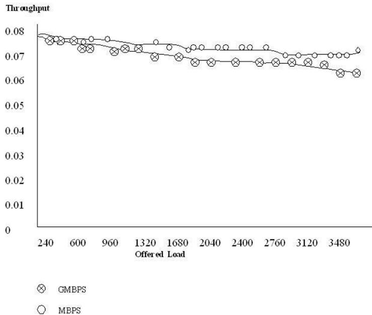
Fig. 3.(c) Graph showing the comparison of Guarded and Non Guarded schemes for Throughput in the three switch ATM network
