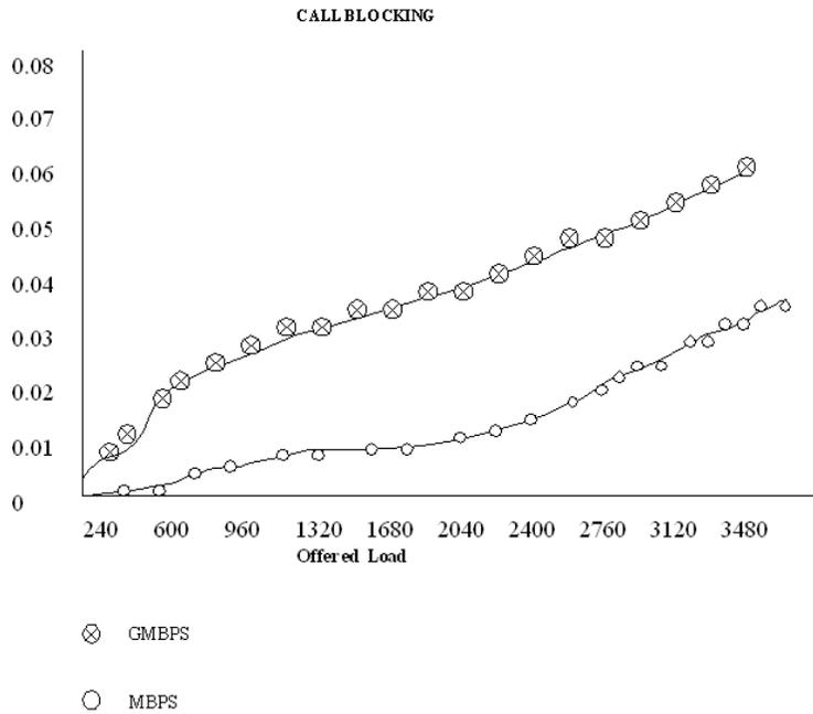
Fig. 3. (a) Graph showing the comparison of Guarded Scheme and Non Guarded Scheme for Call Blocking in the three switch ATM network.
