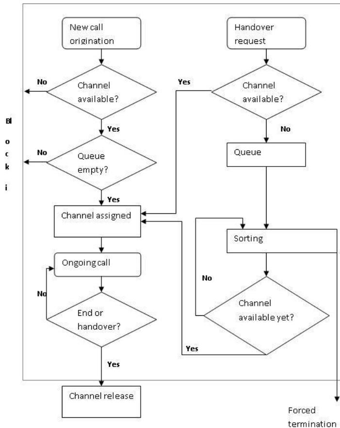
Fig. 2. Call Flow Diagram for the Measurement Based Prioritization Scheme [21].
