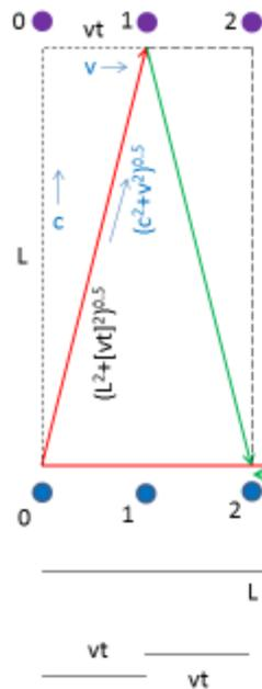
By symmetry, from time step 1 to 2, the two rays (red and green) are reflected back to the source mirror over another time "t." The perpendicular ray covers the same distance at the same speed. However, the horizontal ray now covers a shorter distance  $(L+vt-2vt = L-vt)$  at a slower speed  $(c-v)$ . Since the time "t" is equal in both directions for each time step, we can express it as follows (time = distance/speed):
