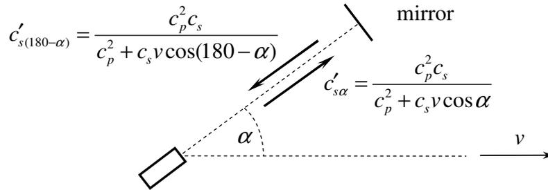
Fig. 25. The velocity of light in the Michelson-Morley experiment
