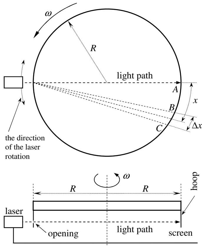
Fig. 56. The measurement system of the velocity of light in one direction
