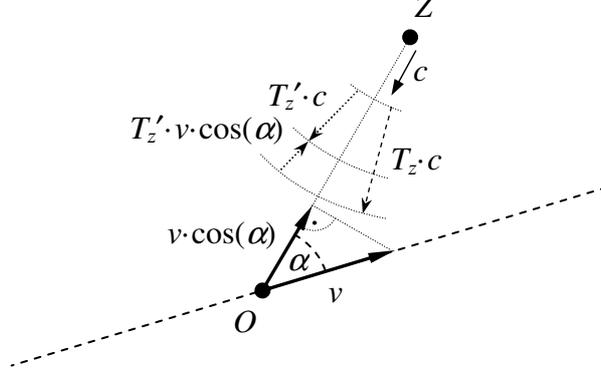
Fig. 78. Observer  $O$  moves relative to light source  $Z$
