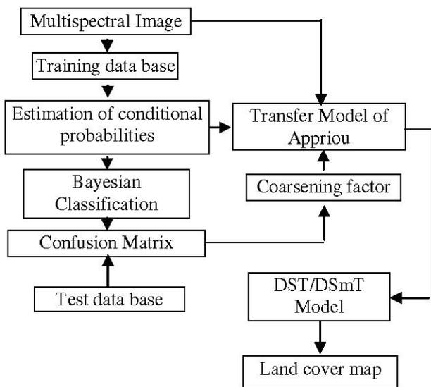
Figure 1. The proposed DST and DSMT classification methodology
