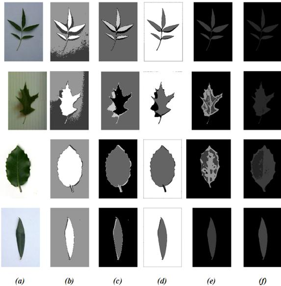
Fig.9. Segmentation results of Scan-like images, (a) the original images, (b) MPZ 1 channel, (c) MPZ 3 channel, (d) Neutrosophic sets, (e) entropy, (f) multi-level thresholding.
