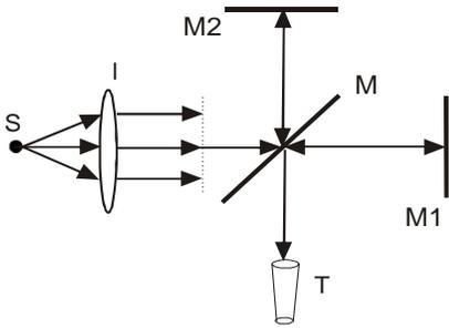
Figure 11 – Michelson-Morley experiment with one semi-transparent mirror, 2 mirrors, a lens and a telescope.
