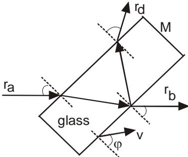
Figure 8 - Semitransparent mirror  $M$  with velocity  $V$  as well as, incident ray ( $r_a$ ), the refracted-reflected ray ( $r_d$ ) and refracted-refracted ray ( $r_b$ ).
