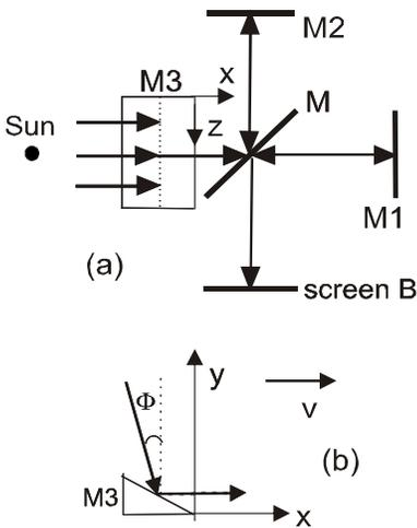
Figure 12 – Michelson-Morley experiment with sun light and screen B. Panel (a) shows the x-z plane, while (b) shows the x-y plane.
