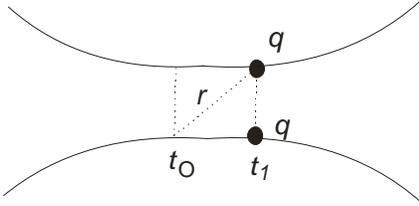
Figure 6 – Trajectories of the two particles  $q$ . In the time interval time  $t_o$  to  $t_1$ , the trajectories are approximately parallel.
