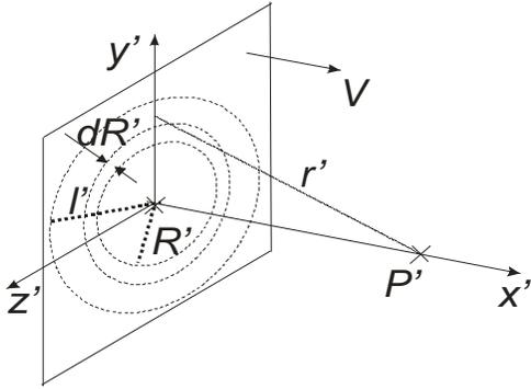
Fig. 3 – Electric field of a uniformly charged plane at point  $P'$  at rest in  $S'$
