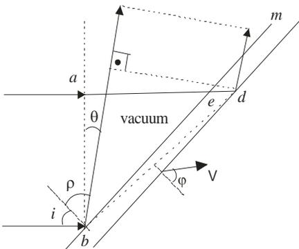
Fig. 9 – Reflection in vacuum. Incident and reflection plane waves
