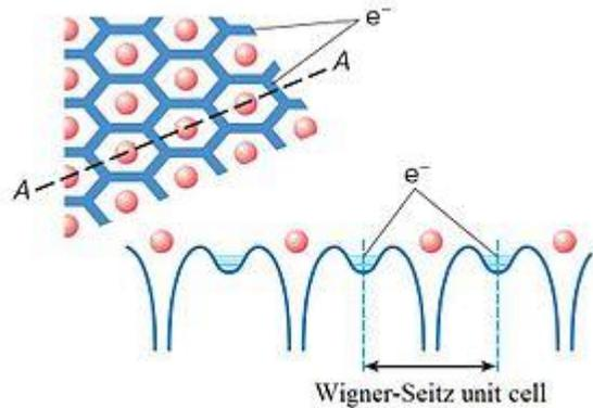
Fig.1 Schematic of valence electron distribution in a Rydberg matter made of excited ( $n=10$ ) Cs atoms
