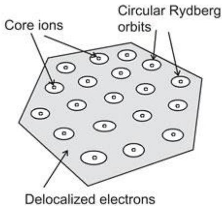
Fig.2 A 19-atom planar Rydberg matter cluster. At the seventh excitation level, spectroscopy on  $K_{19}$  clusters showed the bond distance to be 5.525 nm.
