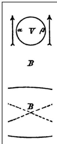
This situation can be explained simply by admitting that the full line is in fact the magnetic wave: when the gap (G) of the circular wire detector is towards the wall (labeled  $\alpha$  in figure) or away from the wall (labeled  $\beta$  in figure) you have a spark because electromagnetic induction is stronger on the side L of the circular wire detector where it is not interrupted by the gap.
