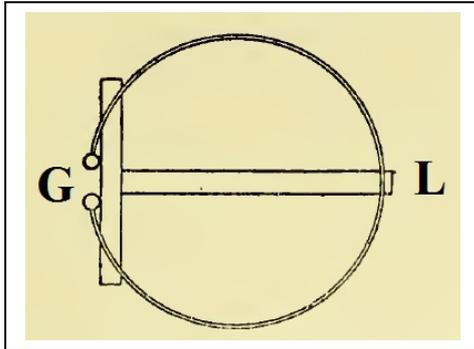
Also, to enable him to easily manipulate the wire circle detector and place it in different positions in space, Hertz mounted it on a T-wooden frame, as shown on the left. The gap (G) and the opposite side (L) are labels to be referred to later as Hertz used them to describe the orientation of the detector in space and thus to claim to be able to detect the electric and magnetic components of the wave.
