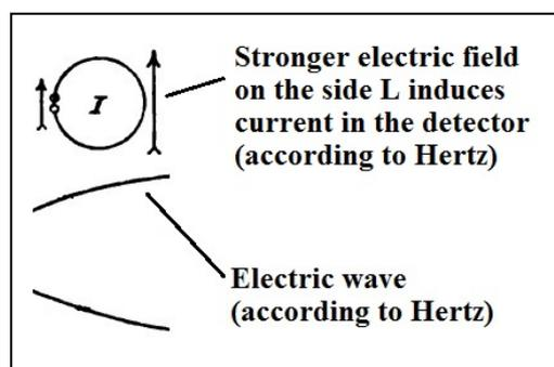
he says that the electric current responsible for the spark at the gap (G) is produced in the circular wire by the electric field of the stationary wave supposedly existing in air; the amplitude of the electric field of the wave is greater on the side (L) opposite to the gap and weaker at the side (G) of the gap, as shown by arrows.
