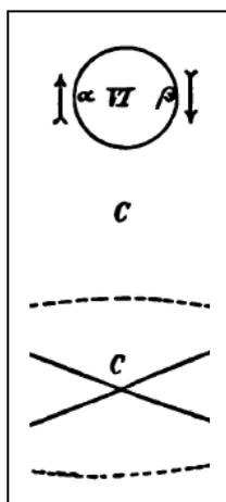
The situation can be explained in the same simple way, consistent with point a): when the gap (G) of the circular wire detector is towards the wall (labeled  $\alpha$  in figure) or away from the wall (labeled  $\beta$  in figure) you do not have a strong spark because the amplitude of the magnetic wave (the full line) is small on the side L so the current produced through electromagnetic induction is too weak to produce a spark.
