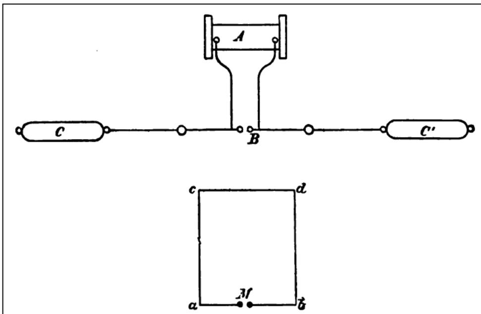
The radio waves were produced by the circuit ABCC' through *spark discharges* at the gap B and were detected with the rectangular wire Mabcd. Hertz's acknowledgement that the *reception of radio waves takes place through the effect of electromagnetic induction* is extremely important because in electromagnetic induction an electric current is induced in a circuit through a time-varying magnetic field.
