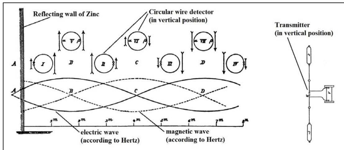
Hertz wrote that in the positions I, II, III and IV he observed sparks at the knobs (gap G) when his detector circle of wire was placed with the gap (G) as shown, sometimes towards the wall, sometimes away from the wall.
