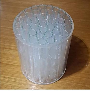
**Figure 12:** By dividing the cup into smaller cylindrical cells, we can displace the oscillation from resonance.
