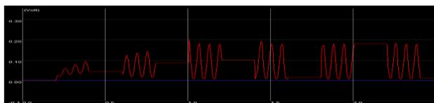
Fig. 3. ASK modulated waveform
