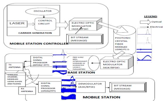
Fig. 1. Radio-over-fiber model for mm-waves
