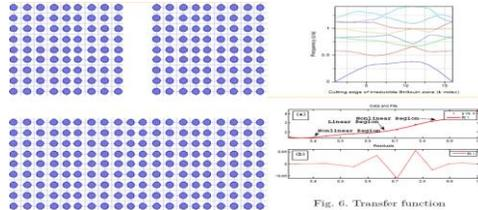
Fig. 5. Photonic crystal amplifier
