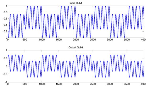
**Figure 9 Input and Output of Hadamard Gate**
