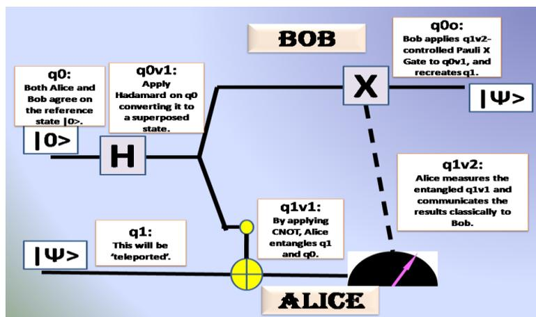
Figure 13 Schematic of 1 qubit quantum teleportation
