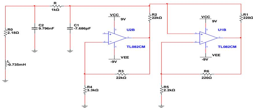
Figure 2 PSPICE Implementation of Chua Circuit using Op Amps
