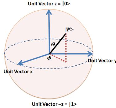
**Figure 5 Bloch Sphere Representation of a Qubit**
