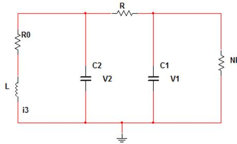
Figure 1 Generalized Chua Circuit
