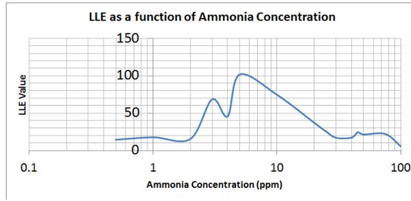
Figure 1: Largest Lyapunov Exponents of the Transient Response as a function of Concentration
