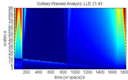
Figure 5: Wavelet Analysis for 50ppm Ammonia Transient Response
