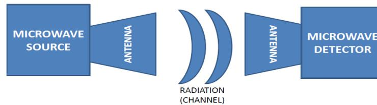
**Figure 1 Block Diagram of the Microwave Material Characterization Setup**
