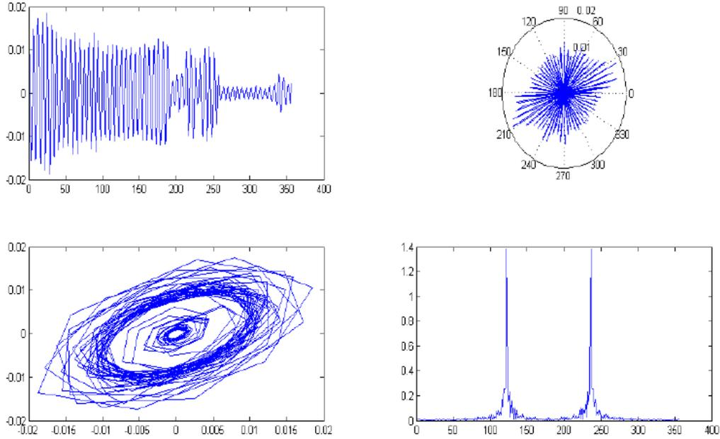
Figure 3 Waveform, Polar Plot, Phase Portrait and Spectrum of Ti/TiO<sub>2</sub> sample, Ti facing Transmitter
