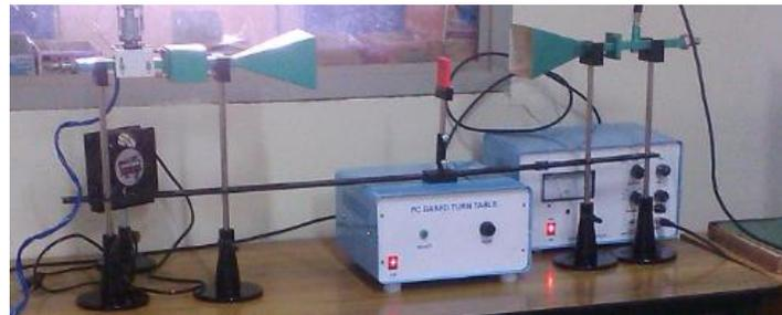
**Figure 2 Photo of the Microwave Material Characterization Setup**
