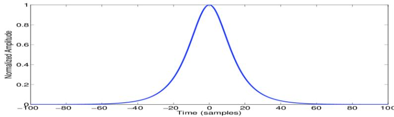
Figure 1 The Hyperbolic Secant Signal
