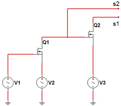
Figure 1: Schematic of two transistor Microwave Chirp Generator
