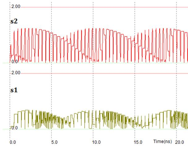
Figure 2: Chirp Generator waveforms of outputs 's2' (Unchirped) and 's1' (Chirped)
