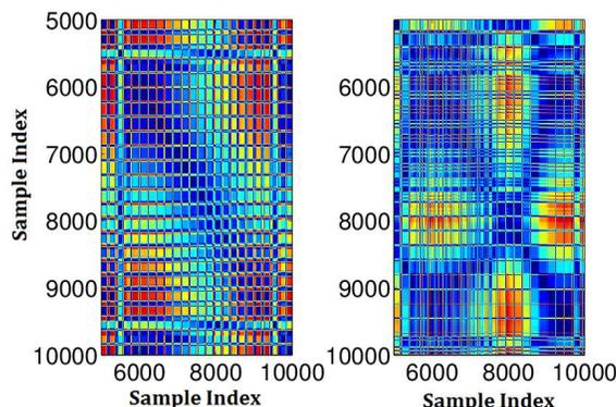
Figure 4: Distance Plots of Unchirped 's2' (left) and Chirped 's1' (right) Signals
