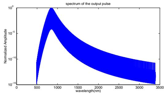
Figure 7: Spectrum of the PCF output with a central wavelength of 850nm
