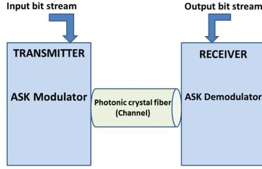
Figure 1: Block diagram of all-optical communication system based on supercontinuum
