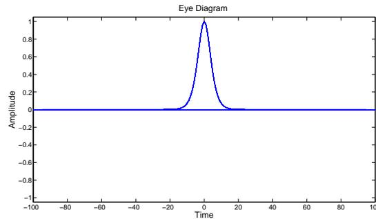
Figure 9: Eye diagram for ultrashort hyperbolic secant based received signal
