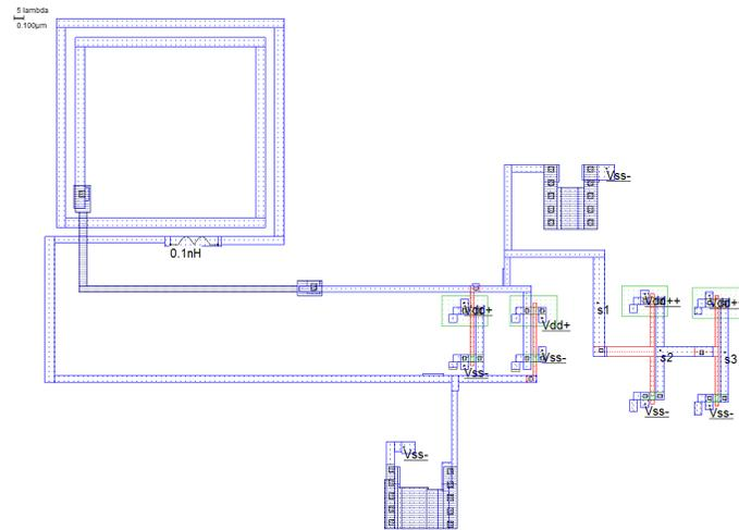
Figure 2: Layout of the CMOS Soliton Generator as obtained from Microwind
