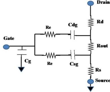
Figure 5: Equivalent circuit of non quasi static channel effect
