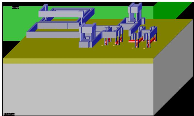
Figure 3: 3D View of the CMOS Soliton Generator as obtained from Microwind
