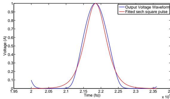
Figure 12: Solitary Wave fitted to square of sech, with a FWHM of 1ps. The output waveform is in blue, and the fit in red.
