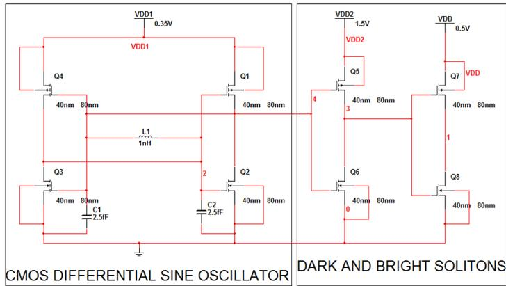
Figure 1: Schematic of the proposed CMOS Soliton Generator consisting of a single inverter
