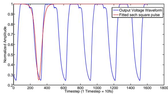
Figure 8: A section of the voltage output of the first CMOS inverter, fitted with a square of sech based pulse, with a FWHM of 1ps
