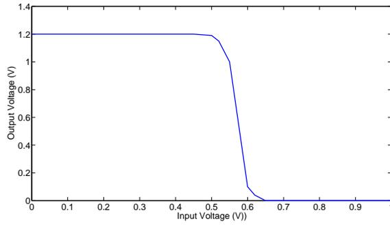
Figure 9: Transfer Characteristics of the inverter designed using Microwind
