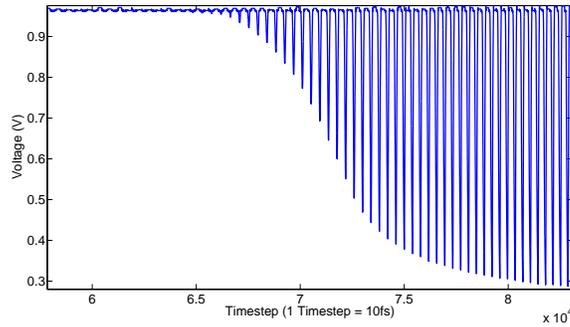
Figure 7: Voltage Output of the first CMOS inverter
