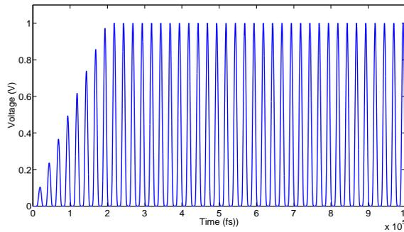
Figure 10: Final Output voltage waveform, showing bright solitons
