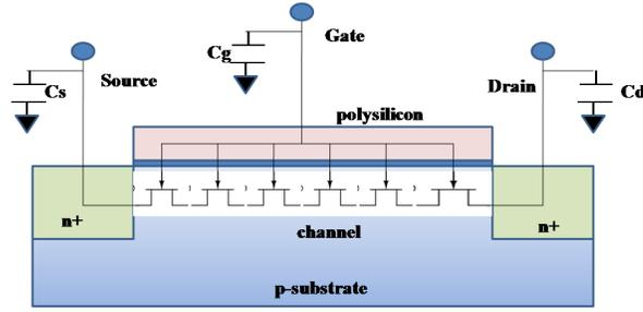
Figure 4: Non-quasi static representation of a NMOS channel
