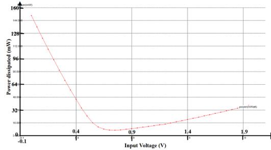
Figure 14: Power dissipated as a function of inverter input voltage, as obtained from Microwind
