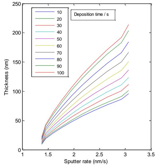
Fig 3: TiN film thickness variation with sputter rate at different deposition time.
