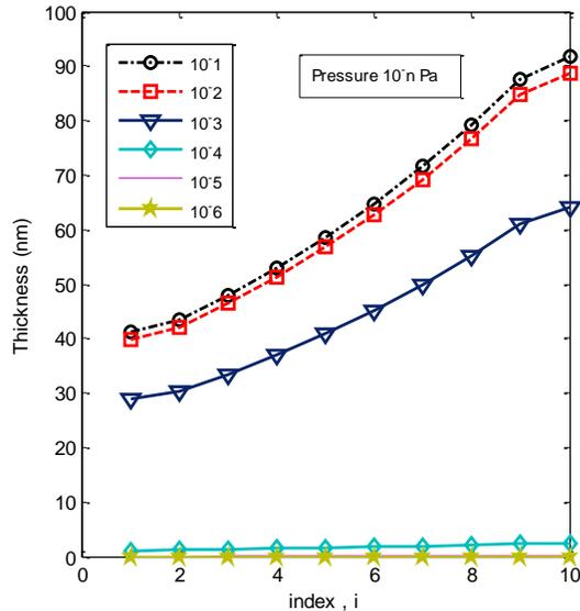
Fig 2: Simulated TiN of various thicknesses deposited at different pressures
