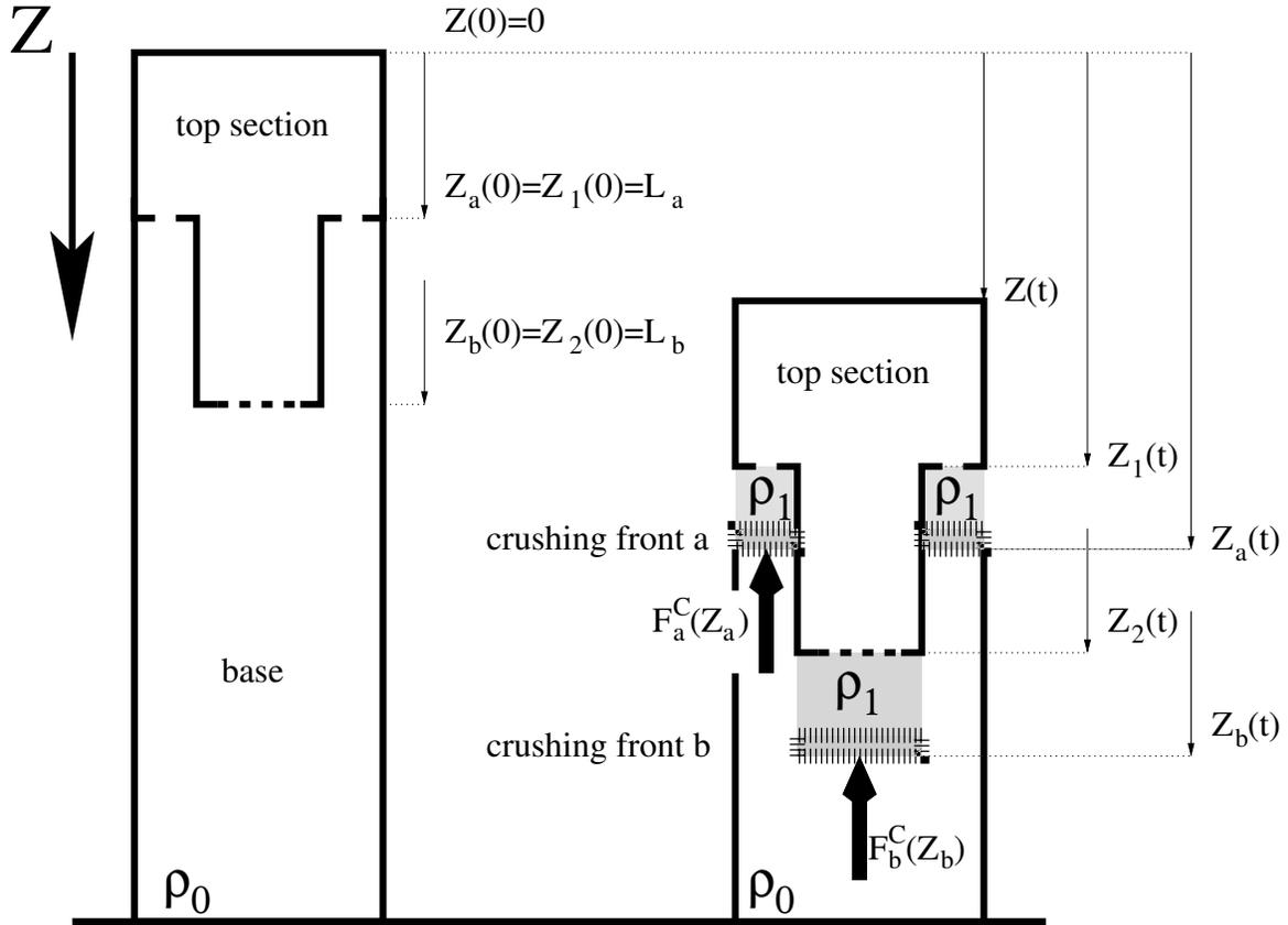
FIG. 2. Schematic of the split-front crush-down model (2.7), which main purpose is to allow us to vary the top section initial mass through separation of crushing fronts at the perimeter and the core of the building. In the NIST hypothesis the crushing fronts at the core and the perimeter are collocated,  $Z_a(t) \equiv Z_b(t)$ .
