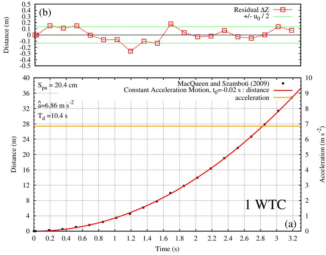
FIG. 1. The best-fit trajectory in the constant acceleration model (2.2). Panel (a) gives the roofline data from Table I (black points), and the model position (red solid line) and acceleration (orange solid line). We also list  $S_{pa}$ , the best-fit acceleration  $\hat{a}$ , and the time  $T_d$  it takes the crushing front to reach the ground. Panel (b) shows the residuals between the model and the data.
