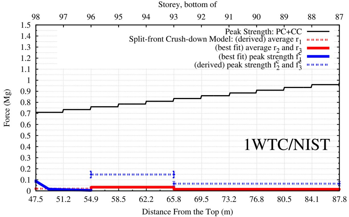
FIG. 3. The NIST hypothesis: Best-fit values (solid red and blue lines) for  $F^C$  (in red) and their averages (in blue) inside the base of 1 WTC. We use best-fit derived  $\epsilon^C$  to estimate one (shown as dotted line of respective color) from the other. We also show the estimated peak strength of the core and the perimeter columns (CC and PC, in black). We see no agreement between the estimated peak strengths of the PC and CC, and their best-fit values.
