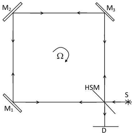
**Figure 6:** a Sagnac interferometer.
