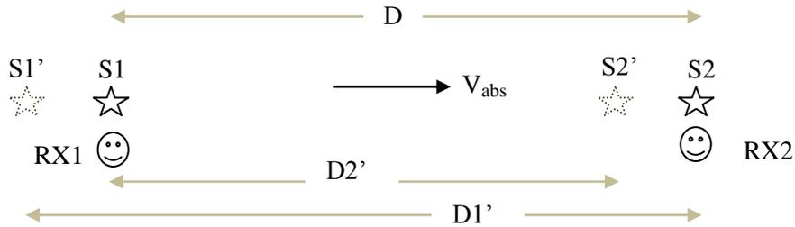
The operation of the clock is as follows: S1 emits a light pulse, then the detector RX2 detects the pulse, S2 transponds with another light pulse without delay, the detector RX1 detects the light pulse and S1 transponds without delay and so on. An electronic pulse counter can count the number of transmissions and hence a clock.
