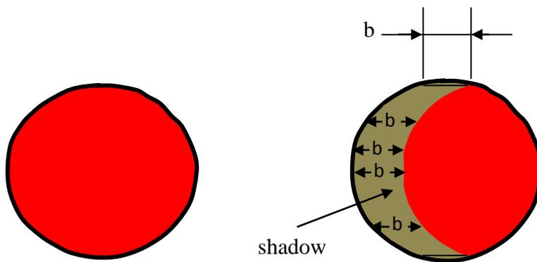
The left diagram shows a bright circular spot on the photo detector which will occur when there is no bending of the light ray. The right diagram shows what the spot of the light ray on the photo detector looks like, with a shadow due to bending of the light ray. Note that the size of the shadow has been exaggerated, which is actually only about 16.56% of the total area of the circle for an absolute velocity of 390 Km/s of the Earth.
