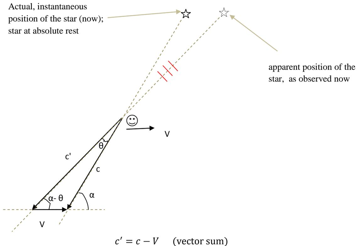
$$\frac{\sin\theta}{V} = \frac{\sin(180 - \alpha)}{c'} = \frac{\sin(\alpha - \theta)}{c} \quad \text{and} \quad \sin\theta \approx \theta \quad (\text{for small angle } \theta)$$
