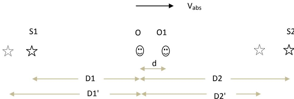
S1 and S2 are satellites, O represents control and monitoring station, O1 represents a GPS receiver. We assume that all clocks are perfectly synchronized, there is no relative motion between the satellites, the control and monitoring station and the GPS receiver, for simplicity. Our aim is to find the order of magnitude of error in position measurements caused by Earth's absolute motion ( 390 Km/s ).
