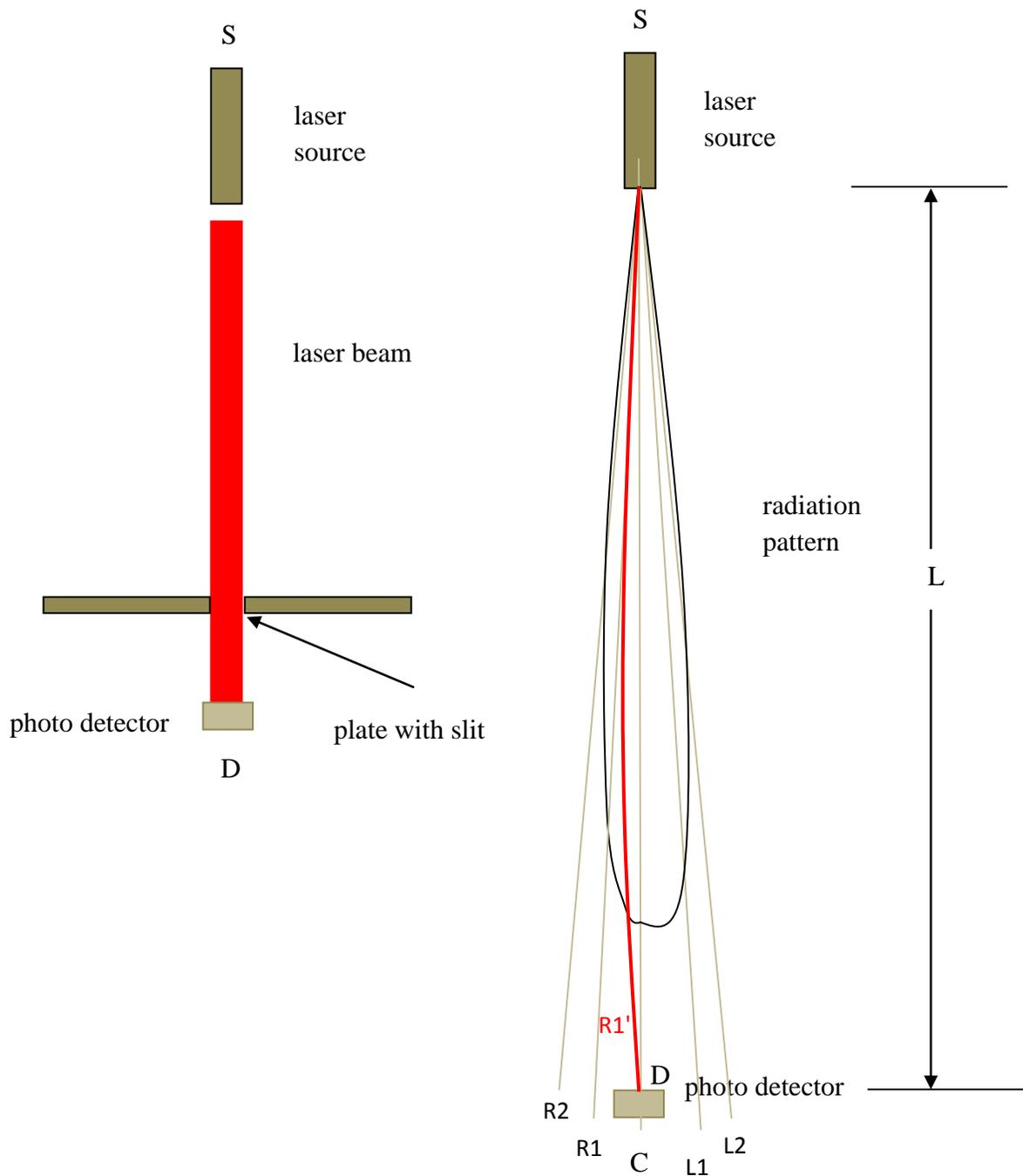
At first assume that there is no plate between the laser source and the photo detector. If the apparatus is at absolute rest and if the laser beam is aligned to the photo detector for maximum light intensity falling on the photo detector, the light ray going to the photo detector in this case will be ray C. Next assume that the apparatus is moving with absolute velocity to the right, without changing the alignment of the laser beam. In this case it will be light ray R1 that
