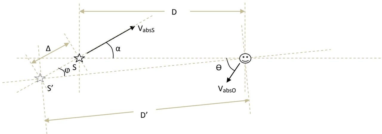
$$(\Delta \cos\alpha + D)^2 + (\Delta \sin\alpha)^2 = D'^2 \quad \dots \dots \dots (1)$$
