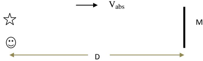
The light source emits a short light pulse towards the mirror. The reflected light is detected by the detector, which triggers the light source to emit another light pulse and so on. A counter counts the number of round trips.
