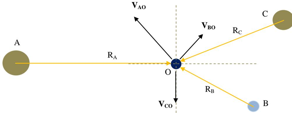
$$V_{absO} = \frac{M_A}{M_T} V_{AO} + \frac{M_B}{M_T} V_{BO} + \frac{M_C}{M_T} V_{CO} \quad (\text{vector sum})$$
