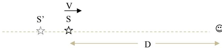
The equations for Doppler effect are the same as above but we see 'aberration' in this case, i.e. the apparent past position ( position of source at the instart of emission ) of source is different from the actual past position.
