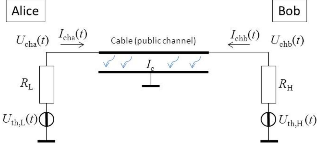
**Figure 7.** The simulated model with LH bit arrangement ( $R_L = 1$  kohm and  $R_H = 9$  kohm).  $U_{cha}(t)$ ,  $I_{cha}(t)$ ,  $U_{chb}(t)$  and  $I_{chb}(t)$  are the voltages and currents at Alice's and Bob's ends, respectively.
