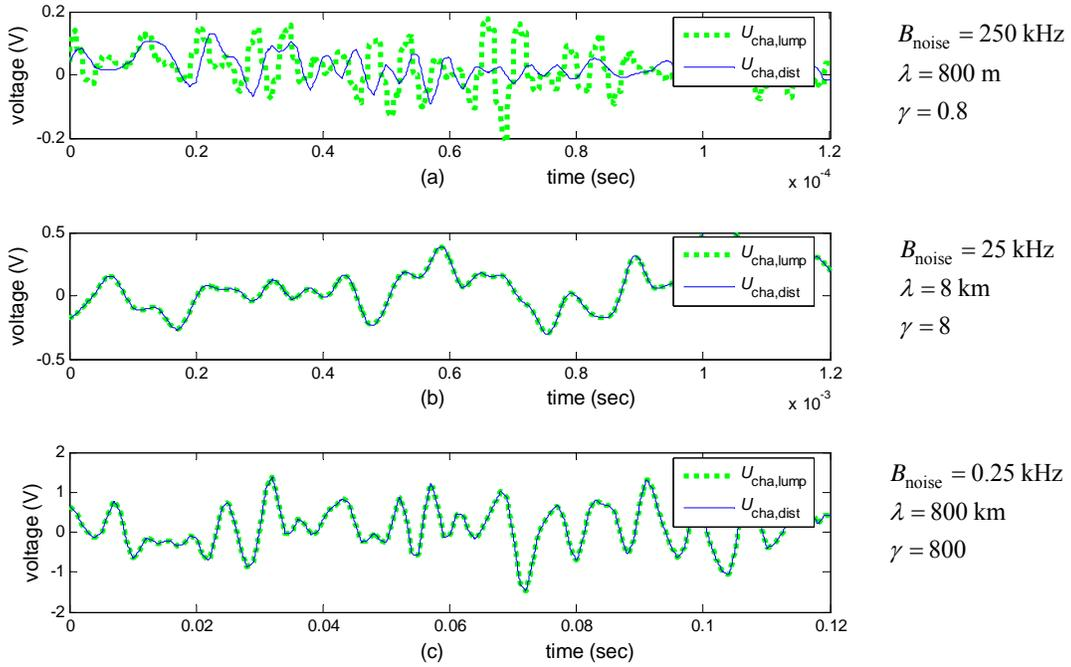
**Figure 6.** The voltage waveforms at Alice's side,  $U_{\text{cha,lump}}$  and  $U_{\text{cha,dist}}$ , for the lumped and distributed element models, respectively, for a 1000 meters cable, at (a)  $\gamma=0.8$ ; (b)  $\gamma=8$ ; (c)  $\gamma=800$ .
