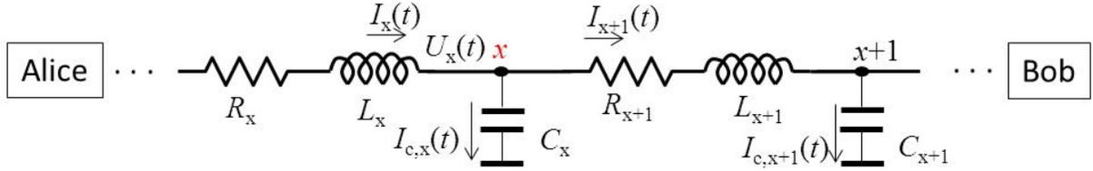
**Figure 2.** Cable model and cable capacitive currents.
