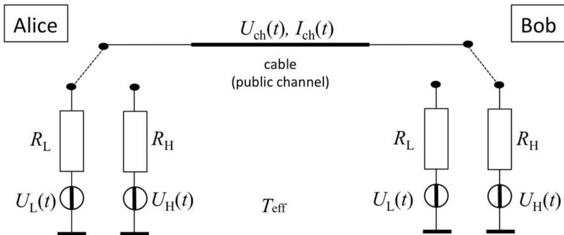
**Figure 1.** The core of the KLJN secure key exchange system [2]. The resistors values are  $R_L$  and  $R_H$ . The thermal noise voltages,  $U_L(t)$  and  $U_H(t)$ , are generated at an effective temperature  $T_{eff}$  (typically  $T_{eff} \geq 10^{14}$  K) [40]. The channel noise voltage and current are  $U_{ch}(t)$  and  $I_{ch}(t)$ , respectively.
