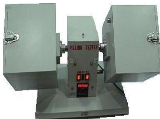
Fig: Digital Pilling Tester
