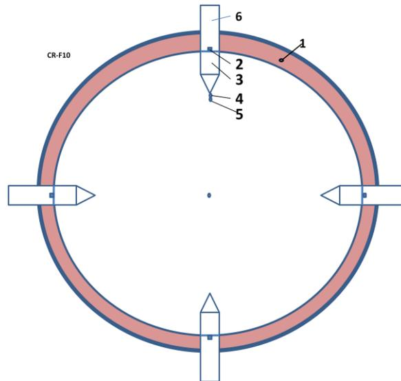
**Fig.4.** Impulse Cumulative AB-thermonuclear reactor (Version 1). *Notations:* 1 – strong sphere, 2 – fuse, 3– explosive, 4 - piston from heavy material, 5 – capsule (pellet) of nuclear fuel; 6 – tube for loading and additional initial acceleration.
