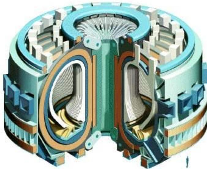
Fig. 2. Magnetic thermonuclear reactor. The size of the installation is obvious if you compare it with the "Little Blue Man" inside the machine at the bottom. Cost is some tens of billions of dollars.
