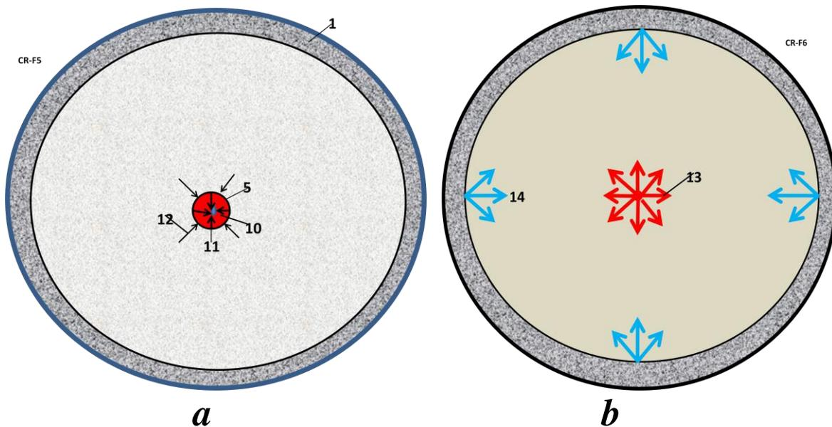
**Fig 9.** Work of Cumulative AB thermonuclear reactor(Version 2). *Notations:* *a* – final of a fuel compression, *b* – thermonuclear explosion and injection of work and cooling liquid (for example, water). 10 is heavy piston (one is in final presses), blocks fuel and increases time for nuclear reaction; 11 - brake pressure; 12 – outer pressure (shock wave from explosive); 13 – thermonuclear exposure of fuel; 14 – injection of a work and cooling liquid (for example, water after MHD).
