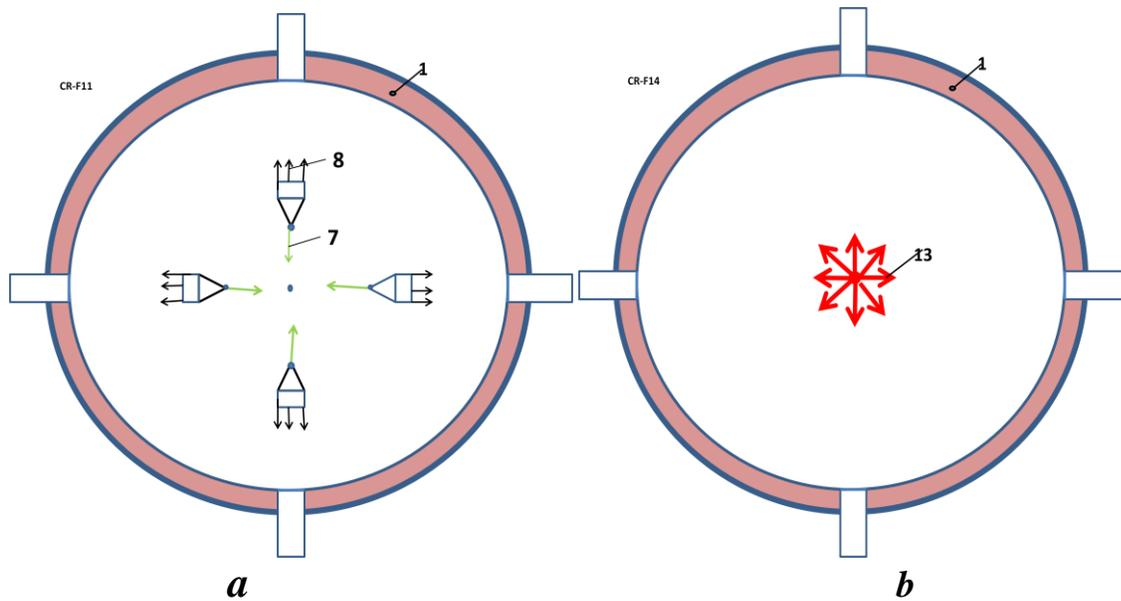
**Fig. 5.** Work of AB thermonuclear reactor (Version 1). Notations: *a* – rocket acceleration of pistons, *b* – nuclear explosion; 7 is moving of explosive and pistons (force from rocket thrust), 8 is flow of rocket explosive gas. 13 – Thermonuclear explosion.
