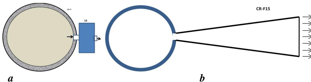
**Fig. 6.** Final (industrial) work of Cumulative AB thermonuclear reactor. Compressed gas from sphere runs to the magneto hydrodynamic (MHD) generator and produces electric energy or runs to gas turbine and produces useful work (Fig. 6a). Notation: 14 – conversion of hot gas pressure to electric or mechanical energy, for example, by the magneto hydrodynamic generator (MHD together with condenser), gas (steam) turbine (Fig. 6a) or moving to a rocket nozzle and produces a rocket thrust (Fig. 6b).
