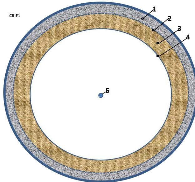
**Fig.7.** Impulse Cumulative AB-thermonuclear Reactor (Version 2). *Notations:* 1 –strong sphere, 2 – net fuse, 3 – explosive, 4 - film (piston) of heavy material, 5 – nuclear fuel.
