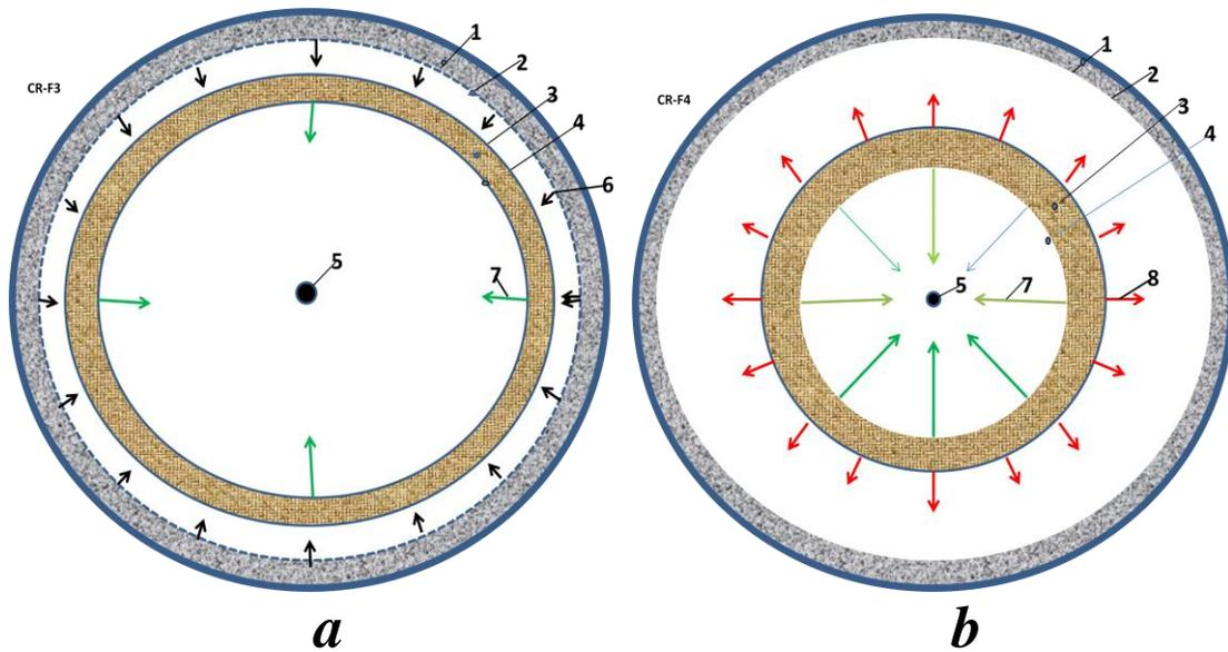
**Fig. 8.** Work of Cumulative AB thermonuclear reactor (Version 2). *Notations:* *a* – initial layer explosive, *b* – rocket part of explosive. 1-5 are same with Fig.7, 6 is pressure of initial layer of explosion, 7 is moving of explosive (force from jetted gas rocket thrust) , 8 is flow of reactive explosive gas.
