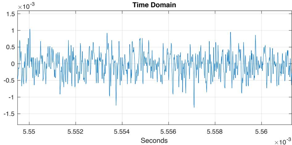
Figure 7 Time Domain Plot (no test signal injection)
