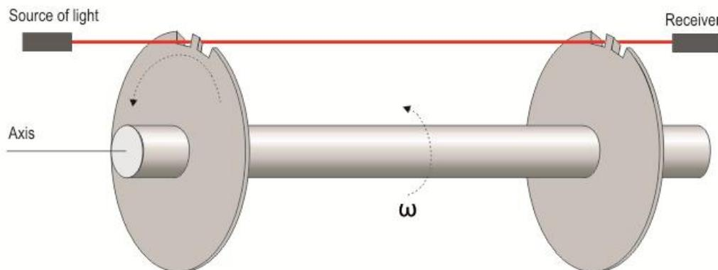
Fig. 1. One way speed of light measurement device with slotted disks, attached to rotating pin.
