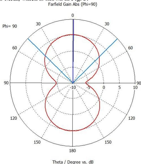
Fig. 3 Gain of proposed Antenna
