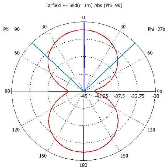
Fig. 4(b). H-field of proposed antenna
