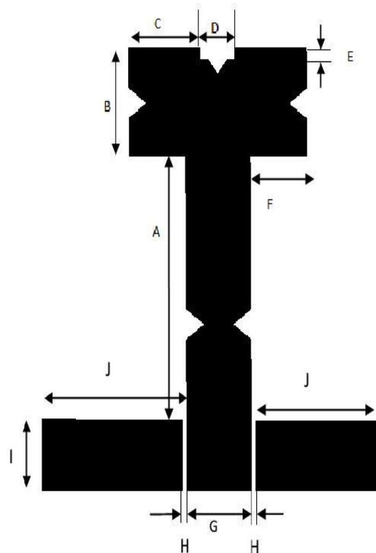
Fig 1. Configuration of anticipated fractal antenna
