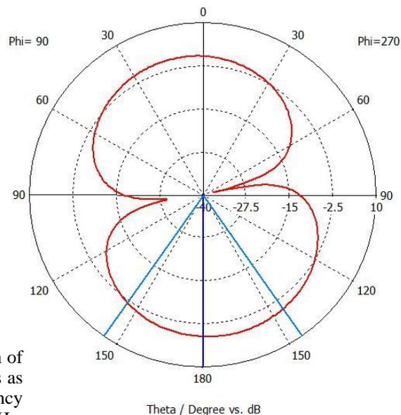
Fig 4 . 2D radiation pattern with frequency 3.4GHz
