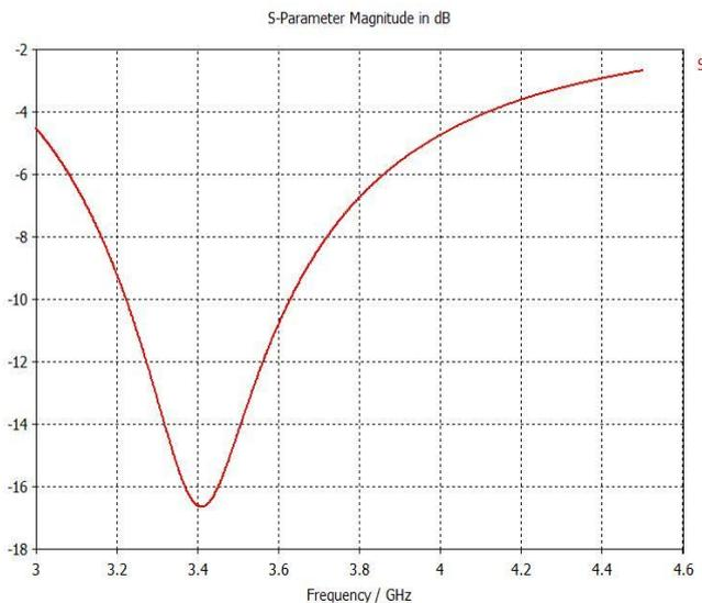
Fig 2. Simulated return loss in opposition to frequency
