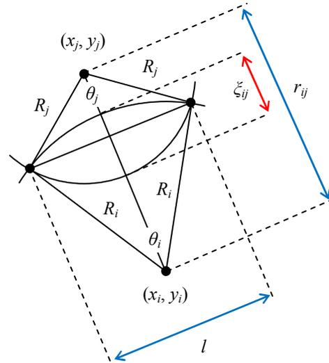
Figure 4. Overlap area between two grains  $i$  and  $j$  with other geometry parameters required for calculation the overlap area.
