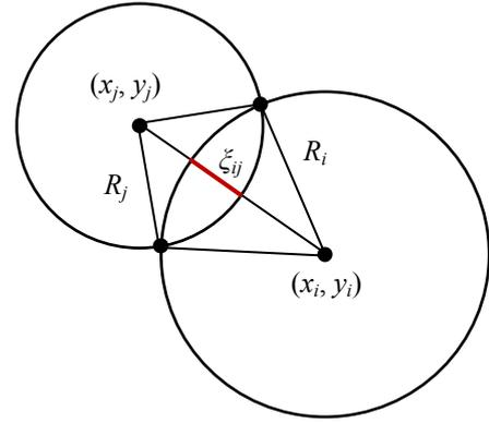
Figure 3. Overlap distance between two spherical grains  $i$  and  $j$ .
