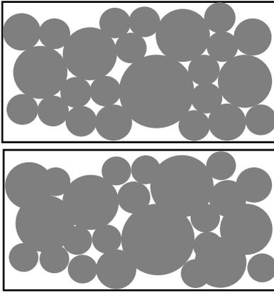
Figure 2. Grains projection on a plane  $z$  for condition: non-overlapping grains (top) and overlapping grains (bottom).
