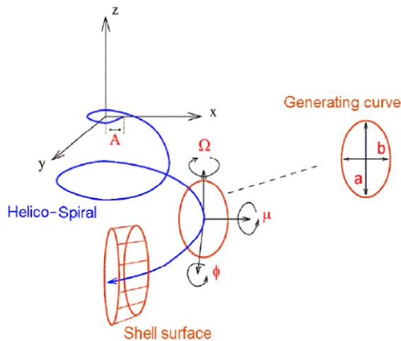
Fig. 2: Illustration of parameters for formed spiral structure. (Courtesy [6])
