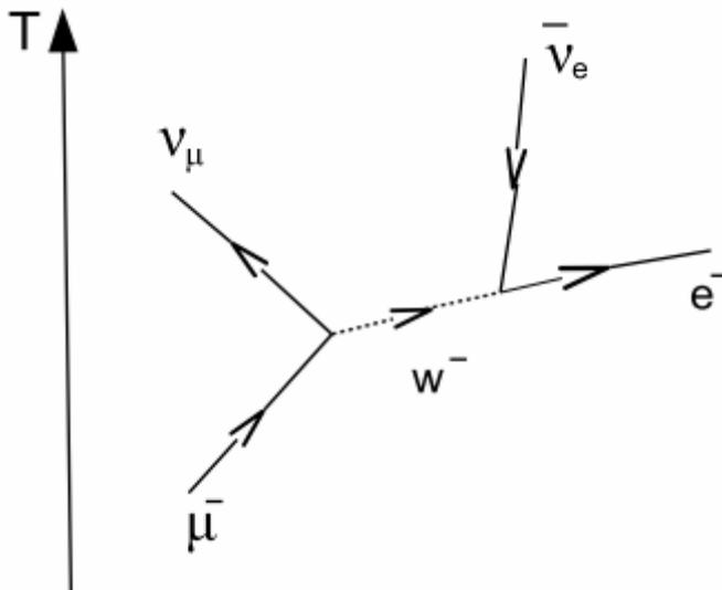
Figure 2. The most common decay of the muon.
