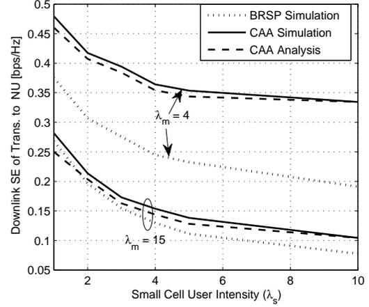
Fig. 8. Downlink SE of transmission to the NU with increase in smallcell user intensity ( $\lambda_s$ ) for different user association schemes (for  $\rho_m = \rho_s = 0$ ).
