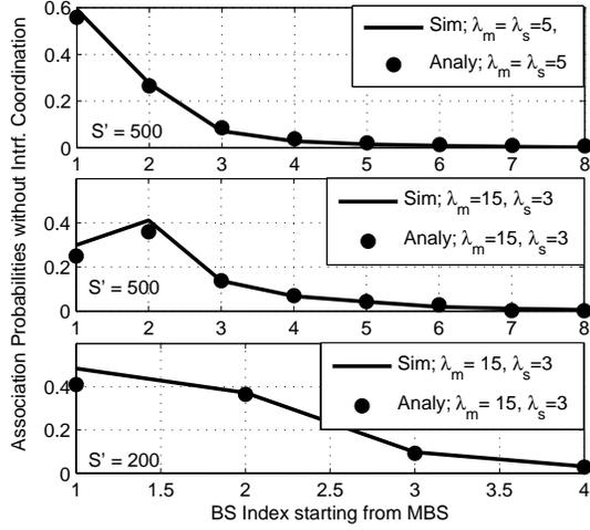
Fig. 3. Association probabilities of the NU with a reference MBS and  $S$  SBSs without interference coordination (for  $R_m = 300$  m,  $T = 100$  m,  $\rho_m = \rho_s = 0$ ). BS indices  $[2, \dots, 4]$  represent the  $S$  SBSs within distance  $T$ .
