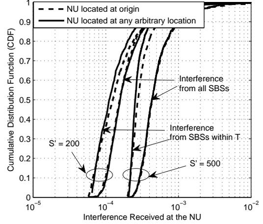
Fig. 5. Comparison of the CDF of the cumulative interference from  $S$  and  $S'$  SBSs considering (i) the exact location of the NU; (ii) NU is located at origin (assumption) (for  $T = 100$ ,  $P_m = 10W$ ,  $P_s = 0.1W$ ,  $\beta = 2.0$ ).
