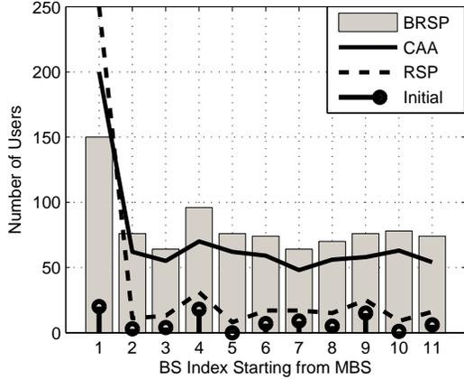
Fig. 7. Traffic load balancing after arrival of 250 NUs in the two-tier smallcell network considering different association schemes (for  $\lambda_m = 15$ ,  $\lambda_s = 3$ ,  $\rho_m = \rho_s = 0$ ).
