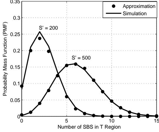
Fig. 2. Comparison between the approximated PMF of the number of SBSs within distance  $T$  given in (19) and the exact PMF obtained from Monte-Carlo simulations (for  $R_m = 300$  m,  $\beta = 2$ ,  $T = 100$  m,  $D_l = 600$  m).
