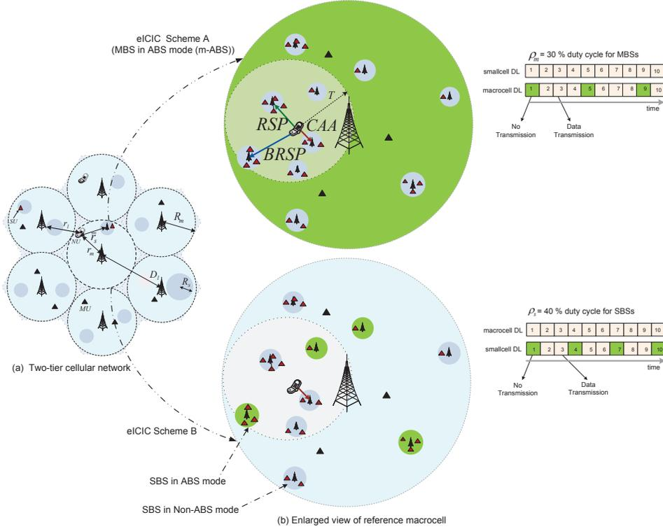
Fig. 1. (a) Graphical illustration of a two-tier smallcell network. In this part of the figure, the distances are demonstrated graphically. (b) Enlarged view of the reference macrocell illustrating eICIC scheme-A for MBS (when MBS is in ABS mode ( $m$ -ABS)) and eICIC scheme-B for SBS (when  $S'_1$  SBSs are in ABS mode ( $s$ -ABS)). Moreover, the working mechanisms of RSP, BRSP, and CAA-based downlink user associations are illustrated.
