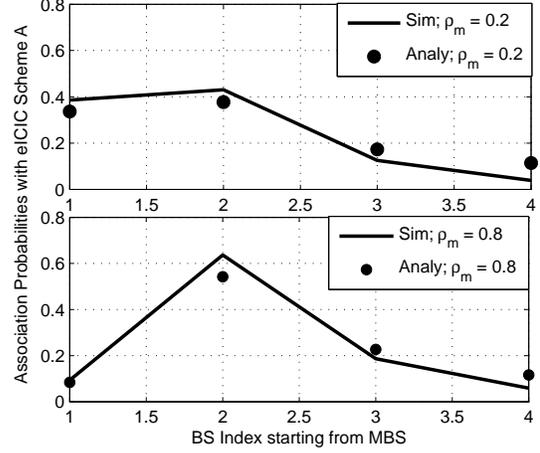
Fig. 4. Association probabilities of the NU with a reference MBS and  $S$  SBSs within distance  $T$  in eICIC scheme-A (for  $R_m = 300$  m,  $T = 100$  m,  $S' = 200$ ,  $\lambda_m = 15$ ,  $\lambda_s = 3$ ). BS indices  $[2, \dots, 4]$  represent the  $S$  SBSs within distance  $T$ .
