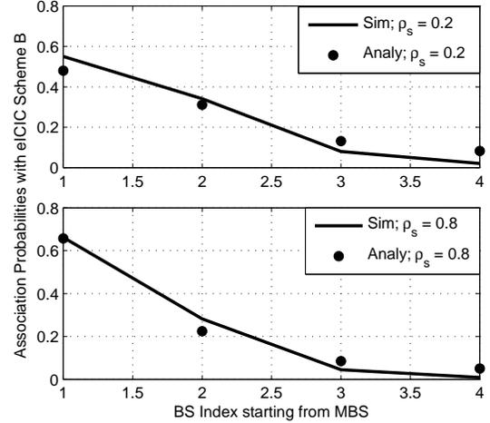
Fig. 6. Association probabilities of the NU with reference MBS and  $Q'$  active SBSs in eICIC scheme B (for  $R_m = 300$  m,  $T = 100$  m,  $S' = 200$ ,  $S'_1 = 100$ ,  $\lambda_m = 15$ ,  $\lambda_s = 3$ ). BS indices  $[2, \dots, 4]$  represent the active SBSs within distance  $T$ .
