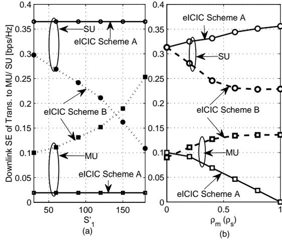
Fig. 12. Downlink spectral efficiency of transmission to MU/SU as a function of (a)  $S'_1$  (for  $\lambda_m = 15$ ,  $\lambda_s = 3$ ,  $\rho_m = \rho_s = 0.8$ ), (b)  $\rho_m$  ( $\rho_s$ ) (for  $\lambda_m = 15$ ,  $\lambda_s = 3$ ,  $S'_1 = 100$ ).
