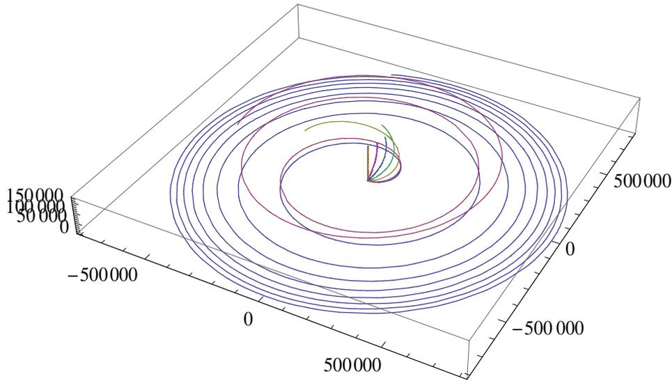
**Figure 5** Plot of signals emanating from O for observer  $O'$  as they rotate with radius  $\rho'$  while advancing in the  $z$  direction for the region  $0 \leq z \leq c/w$  for different values of  $\xi$ . The numbers on the axes are not essential since they depend on the value of  $w$ .
