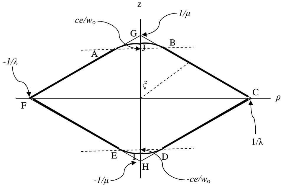
**Figure 10** The diagram in bold lines, AJBCDIEF, describes the locus of points where  $\cos \varphi$  is minimum. The limits ED and AB have been drawn so that  $\frac{ce}{w_0} < \frac{1}{\mu}$ . In the opposite case the diagram is given by the rhombus GCHF. The segments AJB and EID have been drawn arbitrarily as they are the result of the condition  $c^2 - e^{-2(\lambda\rho+\mu z)} w_0^2 z^2 \geq 0$
