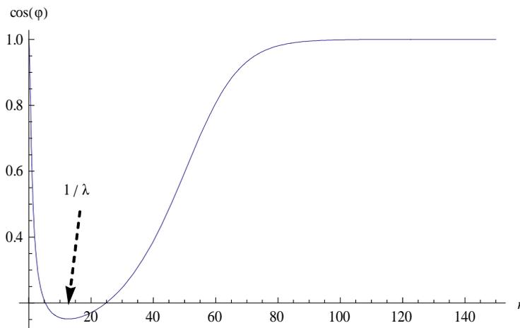
**Figure 9** The cosine of deflection angle  $\varphi$  versus  $r$ . The deflection angle starts at zero ( $\cos 0^\circ = 1$ ). Then it increases reaching almost  $90^\circ$  degrees (for big enough  $w_0$ ) at  $r = \frac{1}{\lambda}$ . Then it falls again to zero ( $\cos 90^\circ = 0$ ) asymptotically.
