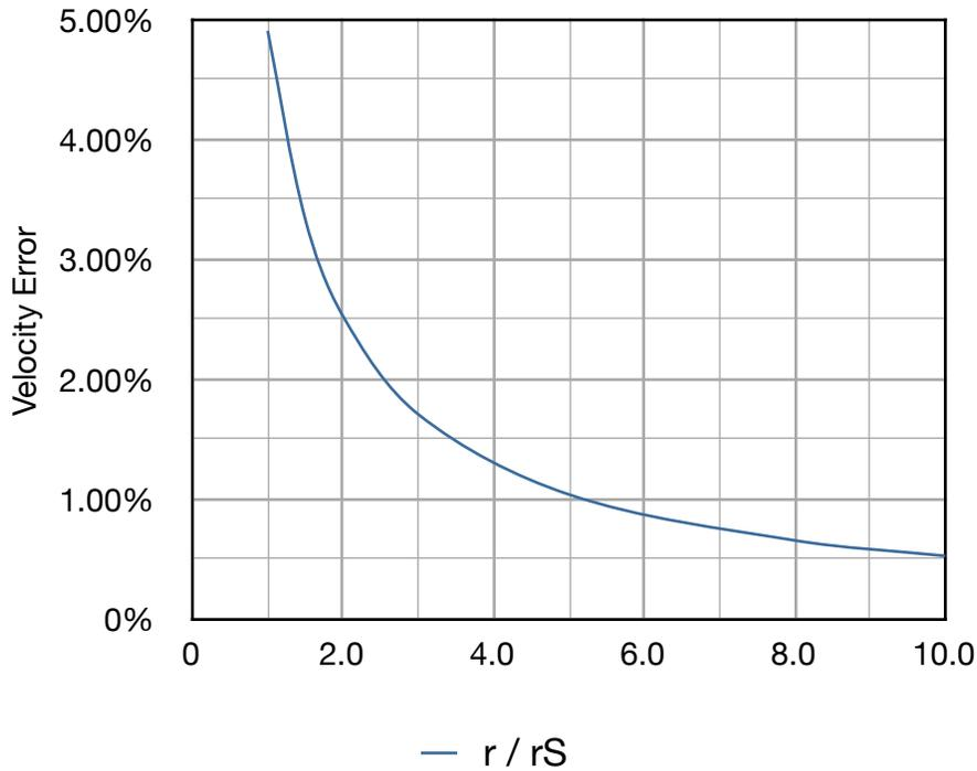
**^ Figure B-1. Velocity Error Introduced by the Square Root Approximation of Equations (B-16), (B-31) and (B-45)**
