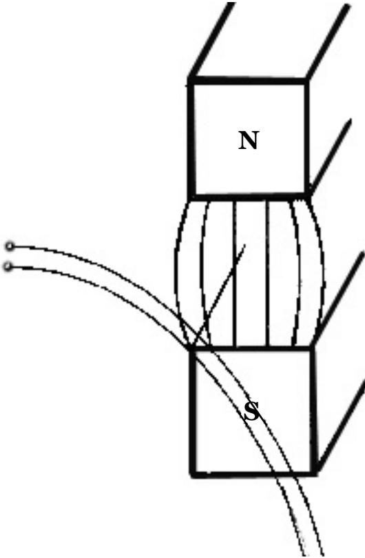
A dipole magnet differs from a normal (bipole) magnet in that two opposite poles are separated by a distance and do not radiate from a common center. Dipole magnets can also be used to manipulate moving electrons and positrons.
