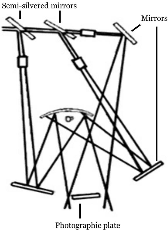
The process of creating a holographic image is complex, involving mirrors, semi-silvered mirrors, beam spreaders etc., to induce the necessary interference patterns. A cup under the curved mirror is holographically photographed onto the plate at the bottom of the picture.
