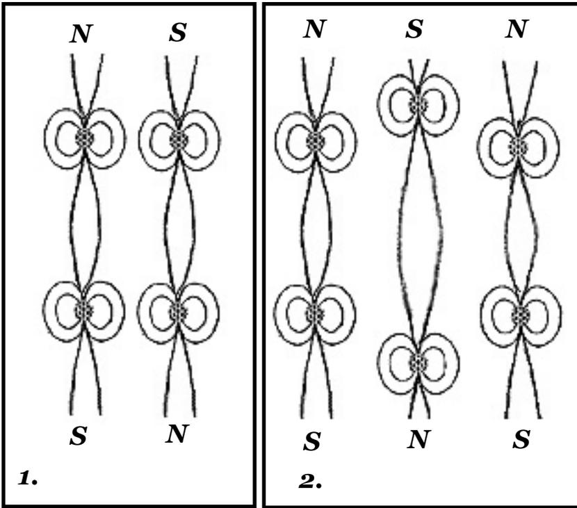
Picture 1 shows antiferromagnetism, the poles of the two lattices are of equal strength and reversed alternately. In picture 2, one possible variation of ferrimagnetism is shown. The center lattice is stretched out and weaker than the ones to either side. Also the poles are reversed.
