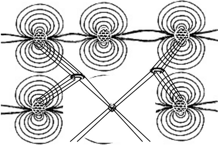
A defect, or missing atom, in the structure of a crystal lattice provides temporary safe haven, or a trap, for a positron.
