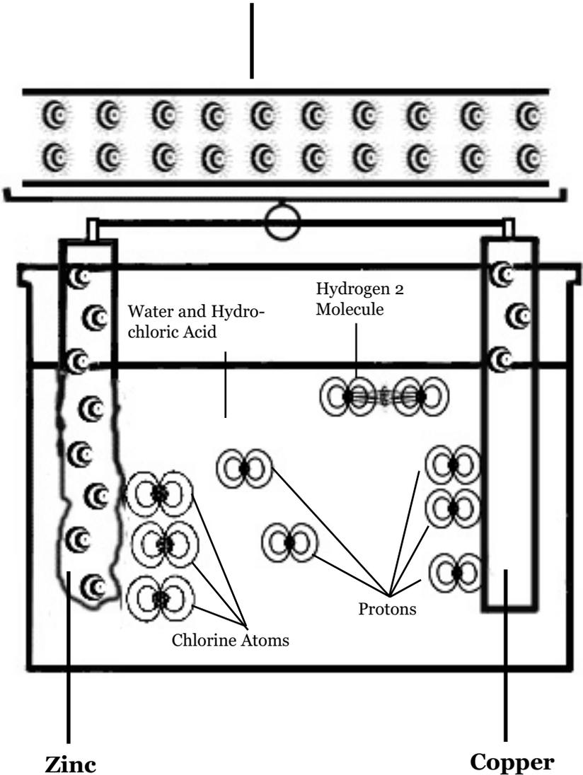
**A simple model of a battery. The protons attach to the copper bar, drawing away electrons as quickly as the zinc bar can release them.**
