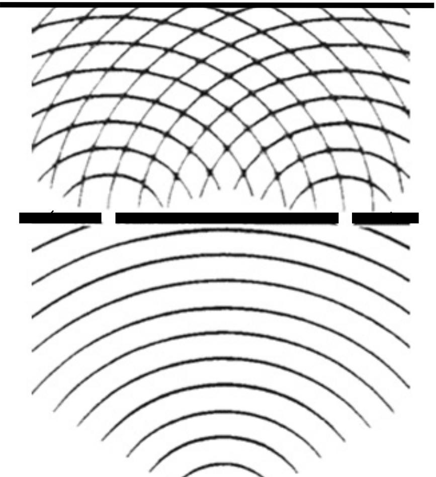
Thomas Young's double slit experiment, proving the wave nature of light by showing interference patterns. It was originally performed in 1801. These experiments allowed Young to first measure wavelengths. In the upper half of the illustration, each intersection can be considered a thermon compressed simultaneously by two waves.
