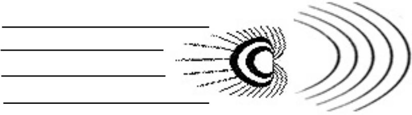
An electron accelerated to near the speed of light, meeting resistance from the EM field and generating synchrotron radiation.
