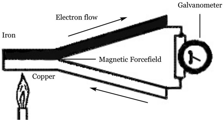
Just as a moving thermal field can move electrons, so electrons can move free and loose thermons. The Seebeck and Peltier effects provide examples of this process. The heat generated by electric resistance provides another example.
