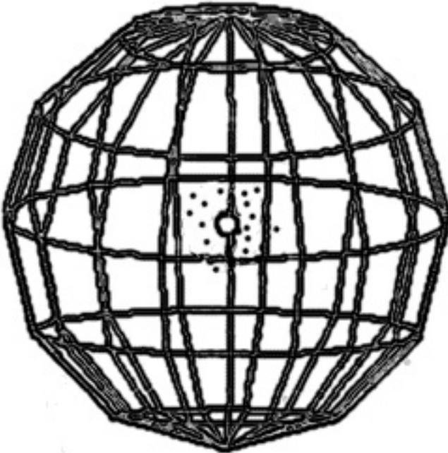
An IEC fusion grid and core. The outer wire mesh acts as an anode surrounding a core cathode. Some experimenters have built these in their homes using “moderately” inexpensive supplies.\*
