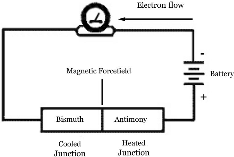
The Peltier effect is also being used in refrigeration and heating devices. A modern single-stage Peltier cooler can lower temperatures to nearly 70 degrees centigrade below room temperature. Peltier coolers have a distinct advantage over conventional refrigerators due to the very localized heat transfer and because they have no moving parts. On the downside, they are less efficient than modern refrigerators and more expensive to operate.
