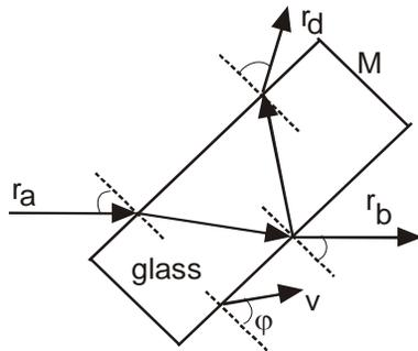
Figure 5 - The semitransparent mirror  $M$  with velocity  $V$ ; the incident ray ( $r_a$ ), the refracted-reflected-refracted ray ( $r_d$ ) and the refracted-refracted ray ( $r_b$ ).
