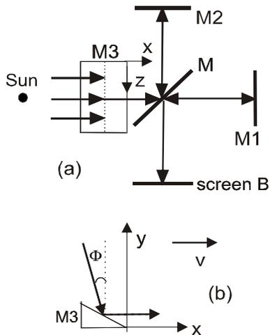
Figure 9 – Michelson Morley experiment with sun light and a screen B. (a) is the plane x-z and (b) is the plane x-y.
