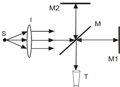
Figure 8 - The Michelson Morley experiment with one semi-transparent mirror, 2 mirrors, a lens and a telescope.
