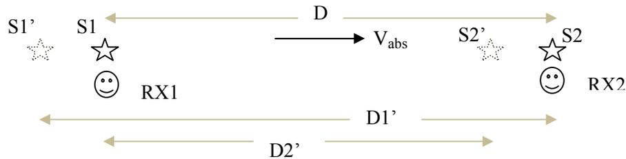
The operation of the clock is as follows: S1 emits a light pulse, then the detector RX2 detects the pulse, S2 transponds with another light pulse without delay, the detector RX1 detects the light pulse and S1 transponds without delay and so on. An electronic pulse counter can count the number of transmissions and hence a clock.
