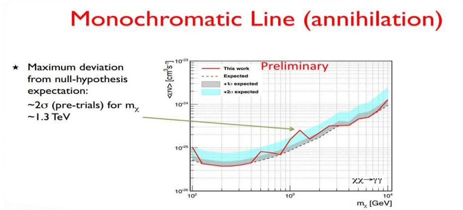
**Figure 1.** Upper limits on  $\langle\sigma_{ann}v\rangle$  for direct annihilation into two photons, as a function of  $m_\chi$ , from the Segue 1 observations with MAGIC (solid line) and as expected for the case of no signal (dashed line), as well as for a signal of  $1\sigma$  or  $2\sigma$  significance (gray and light blue shaded areas, respectively). Figure adapted from [29].
