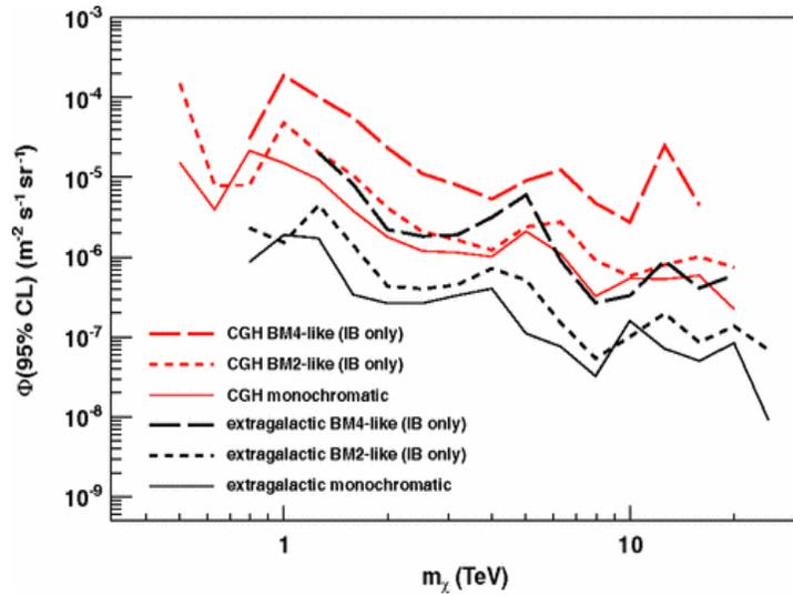
**Figure 3.** Flux upper limits on spectral features arising from the emission of a hard photon in the DM annihilation process. The monochromatic line limits, assuming  $m_\chi = E_\gamma$ , are shown for comparison. Figure adapted from [30].
