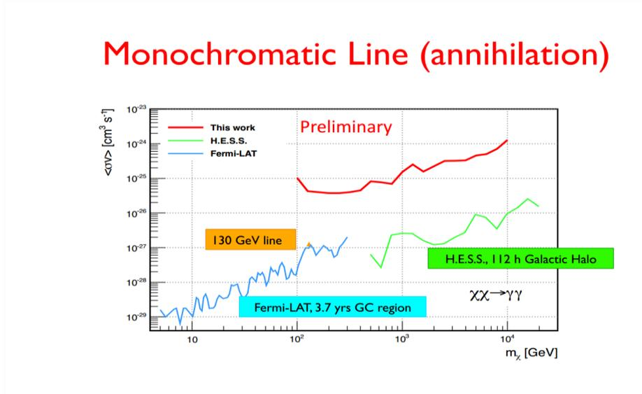
**Figure 2.** Upper limits on  $\langle\sigma_{ann}v\rangle$  for direct annihilation into two photons, as a function of  $m_\chi$ , from the Segue 1 observations with MAGIC and from Galactic Halo observations with H.E.S.S. Figure adapted from [29].
