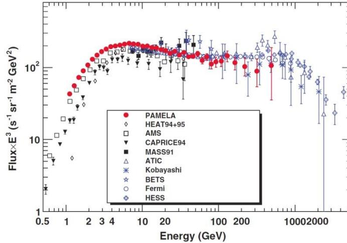
**Figure 5.** The electron energy spectrum obtained in this work (PAMELA) compared with modern measurements: CAPRICE94, HEAT, AMS, MASS91, Kobayashi, BETS, ATIC, HESS, Fermi. Note that the data points, indicated with blue symbols, and the highest data point from HEAT are for the electron and positron sum. The figure adapted from [33].
