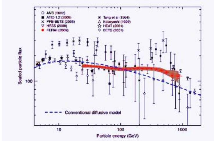
**Figure 4.** The Fermi LAT cosmic ray (CR) electron spectrum (red filled circles). Systematic errors are shown by the gray band. Other high-energy measurements and conventional diffusive model are shown. Figure adapted from [32].
