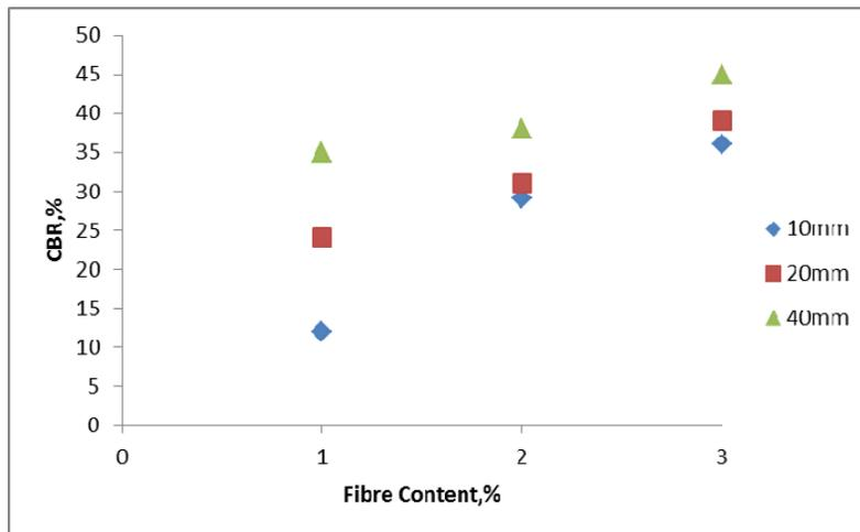
Figure. 6 results of CBR test for natural fibre
