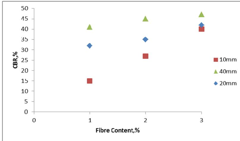
Figure. 5 results of CBR test for plastic fibre
