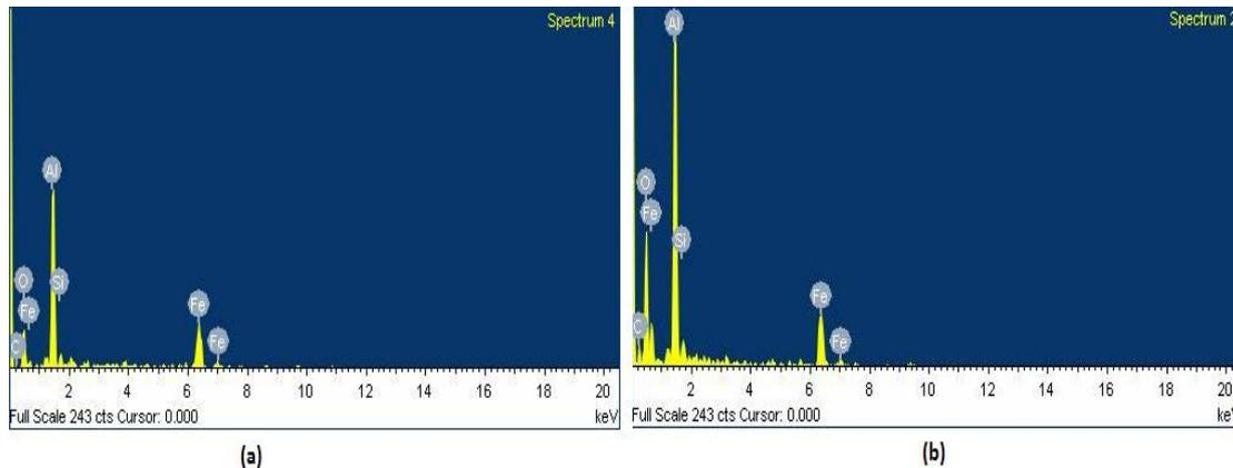
Fig. 13 EDS of wear debris of FSPed sample at locations marked in (Fig. 11)
