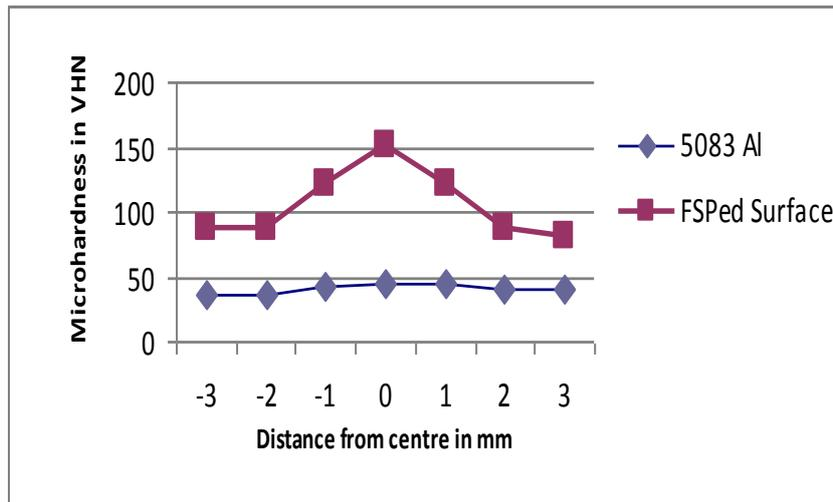
Fig. 5 Hardness profile measured across top surface of the FSPed and unprocessed 5083Al samples
