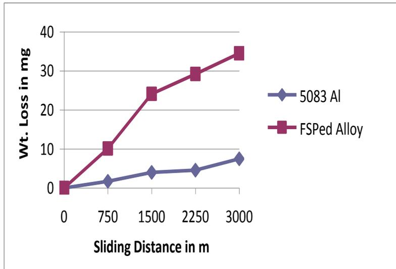
Fig. 7. Variation of weight loss with sliding distance
