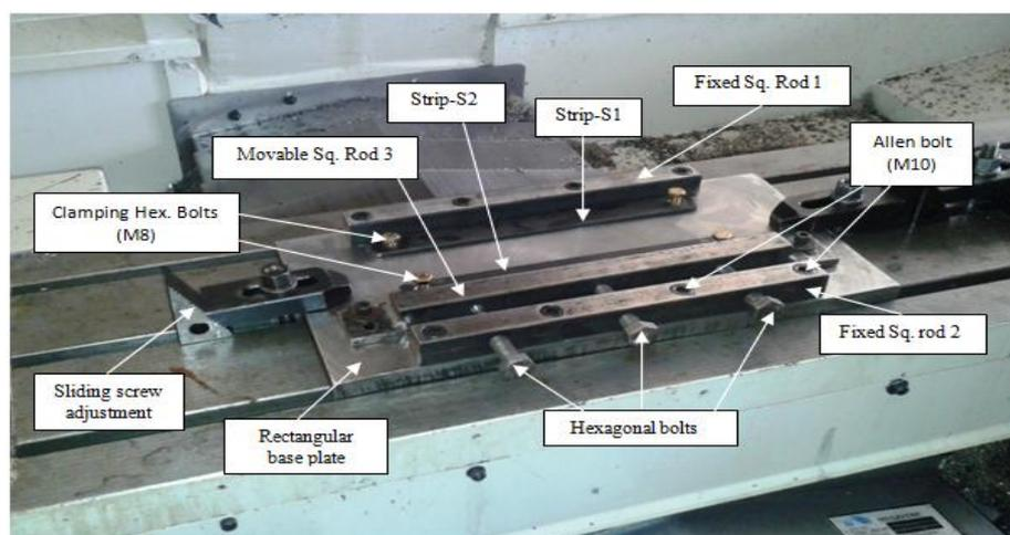
Fig. 1 Fixture for holding specimen during FSP
