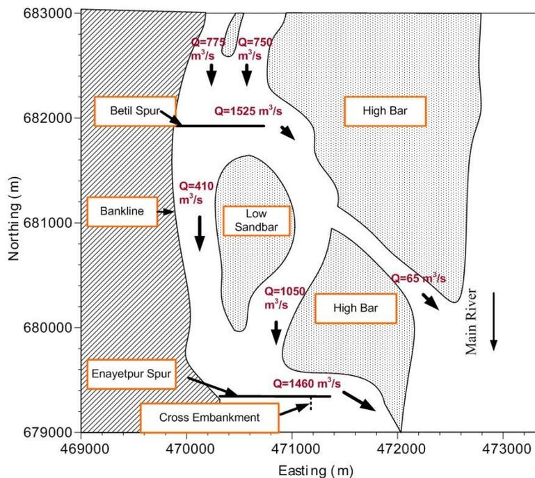
Fig. 7. Discharge of different channels around Betil and Enayetpur spurs
