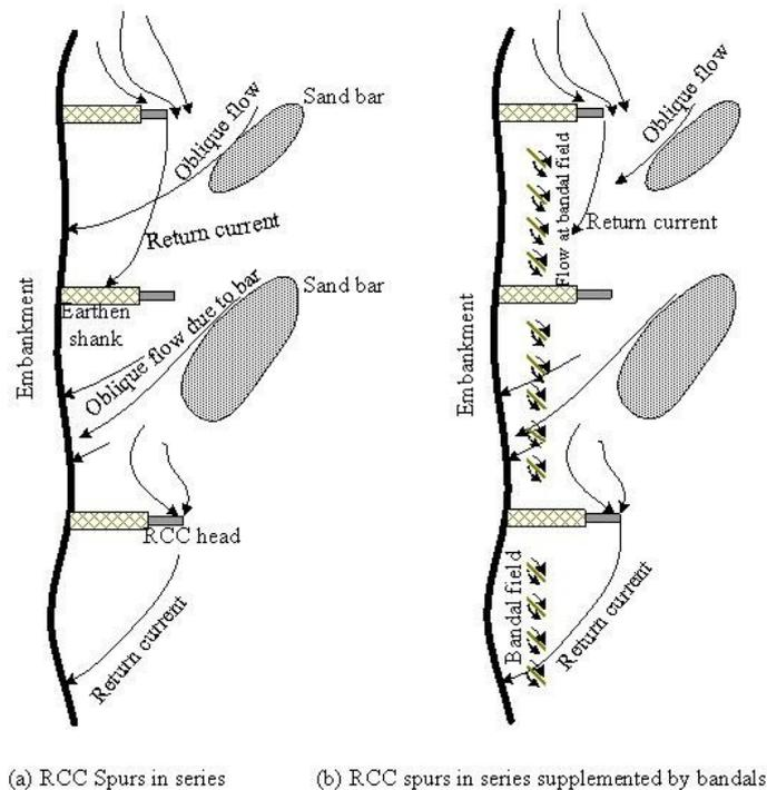
Fig. 17. Conceptual model of bandal-like structures in between RCC spurs
