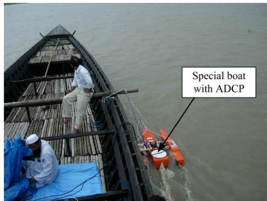
**Fig. 5.** Data collection using ADCP
