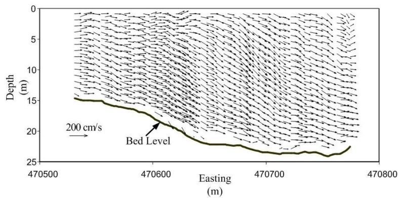
**Fig. 12.** Velocity vectors in the vertical plane around the Betil spur along line b-b
